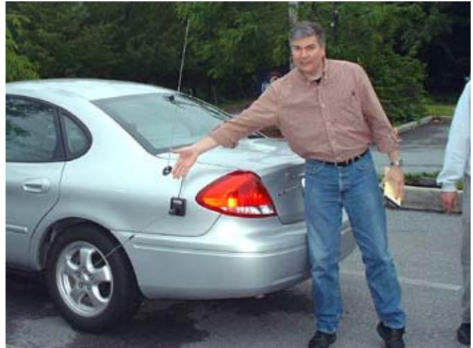
*Mike, N2EAB shows where his mag-mount 2 meter antenna was located for horizontal polarization.*
