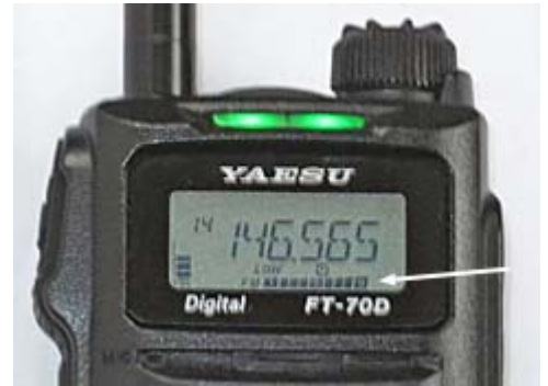
Handi-talkie from a Japanese manufacturer may have more segments on the S-meter (arrowed).
