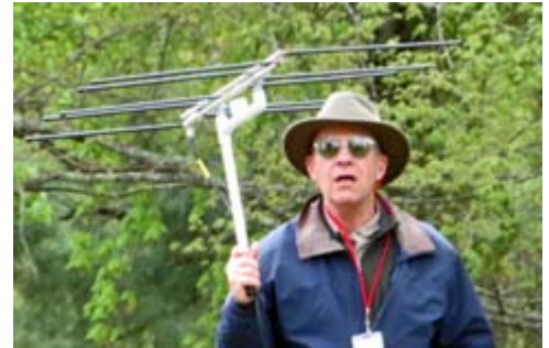
Elk Antennas dual band log periodic antenna in use by David KD2EVI.
