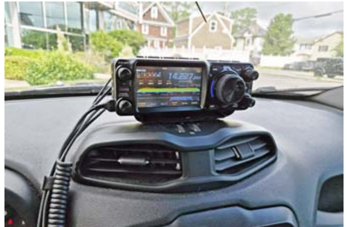
Ray’s Yaesu FTX-1 head unit is now mounted on the dash rather than on the Lido cup-holder mount. [W2CH pics.]
