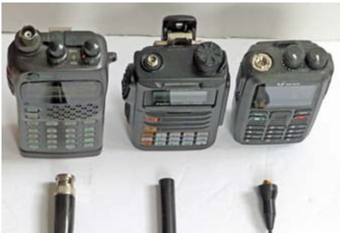
Handi-talkies with their antennas and connectors. L to R: older Icom with male BNC antenna; modern Yaesu with male SMA antenna; BFDX with female SMA antenna.
