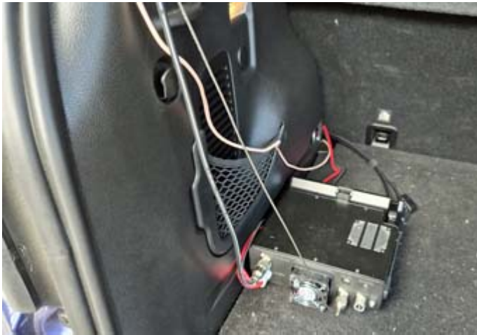
Yaesu SPA-1 amplifier mounted in the trunk of Ray's Jeep.
