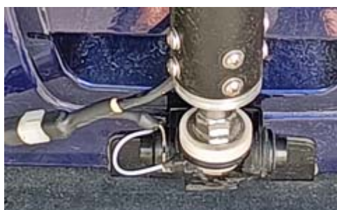
Close-up of Comet trunk-lip mount for the Tarheel antenna.
