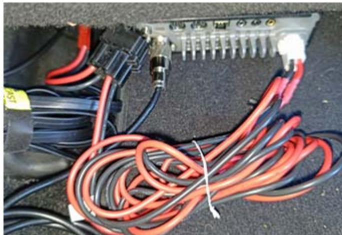
Yaesu FT-891 HF/6m transceiver mounted under the front passenger seat.
