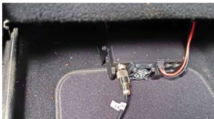
Body of the Kenwood TM-D710GA dual-band FM transceiver mounted under the driver's seat.
