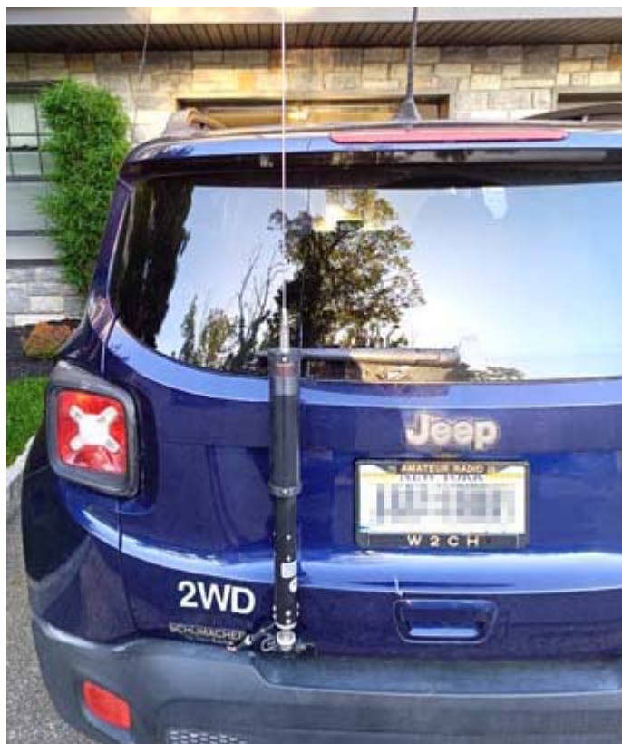
The Tarheel Little Pro antenna mounted on the rear hatch.
