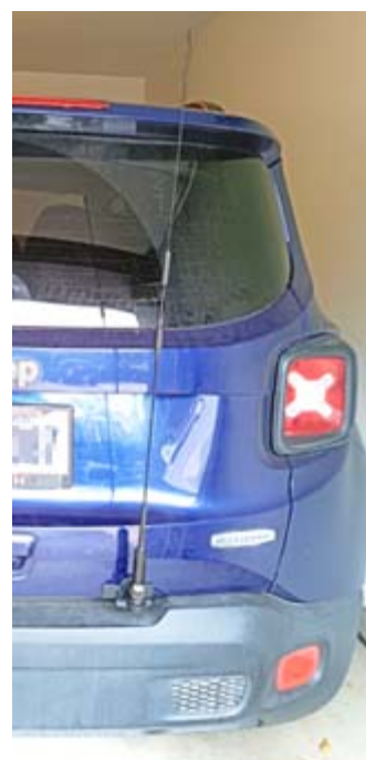
VHF/UHF antenna on rear hatch. [All pics - W2CH].
