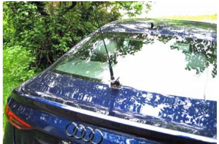
Comet SBB-1 144/440 MHz mobile antenna is fastened to a Comet CP-5M adjustable lip mount. [KD2EVI pic.]
