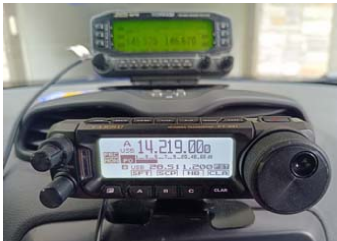
Yaesu FT-891 detachable front panel mounted on the dash in front of the air vents. The VHF/UHF FM transceiver in the background is fastened to the dash with Velcro®.
