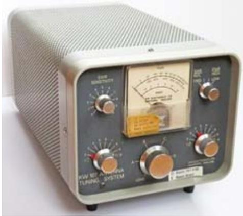
*KW Electronics KW 107 Antenna Tuning System.*
