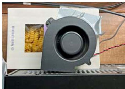
*Additional cooling for Karl's FT-DX1200 transceiver. [N2KZ pic.]*
