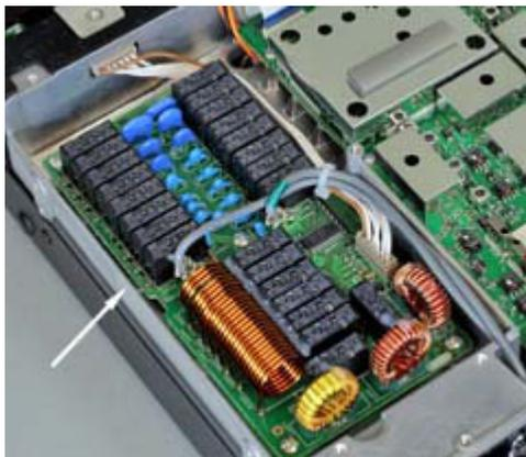
Automatic antenna tuner in Yaesu FT-991 transceiver can match up to a 3:1 SWR.
