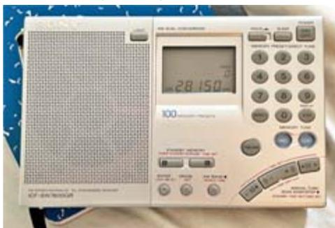
*Sony ICF-SW7600GR portable shortwave receiver for checking beacon coverage. [N2KZ pic.]*
