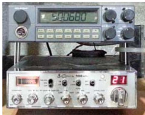
*XE2O/B beacons on 10 meters and 6 meters feature a modified Cobra 148 GTL and a Ranger RCI-5054DX transceiver.*
