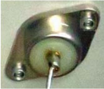
*SO-239 riveted to the painted rear panel of the MFJ-948 tuner.*
