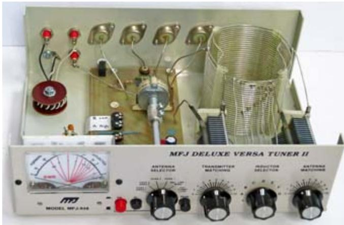
Internal view of the MFJ-948 tuner. Tapped inductor is at top right with air-spaced variable capacitors alongside.
