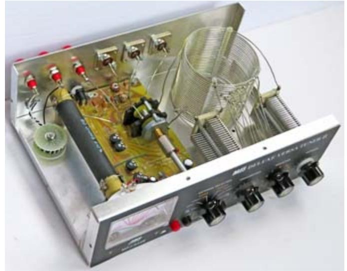
*View inside the MFJ-949E Versatuner. Dummy load resistor is visible at left. Tapped inductor and variable capacitors of the T-network are on the right.*
