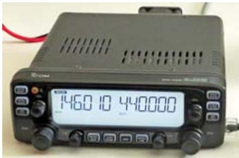
*Icom IC-2730A front panel display after initial power-up.*
