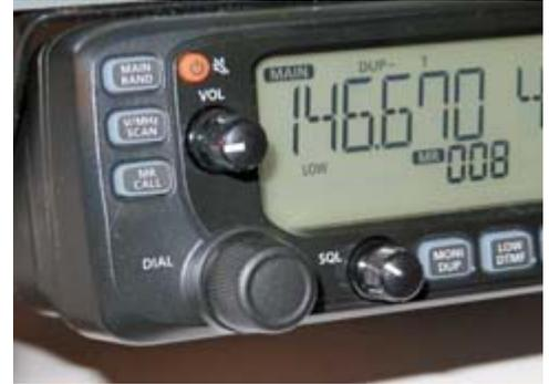
*Positions of volume and squelch control knobs marked with white vinyl tape.*
