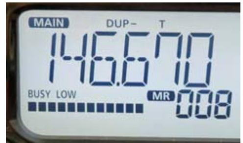
*Close-up of the IC-2730A display showing the 12-bar S-meter below the frequency.*
