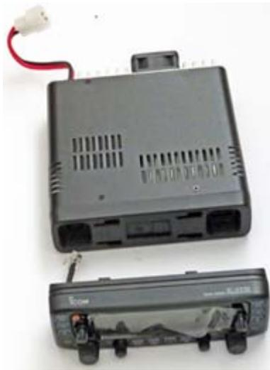
*Attachment of the controller head with MBA-4 bracket onto the IC-2730A main unit*
