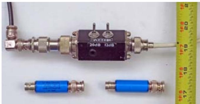
*20dB/12dB switched attenuator was assisted by two more 10dB attenuators, used with the tape-measure Yagi.*
