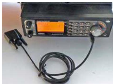
*Uniden BCT15X scanner was supplied with an RS-232 serial programming cable.*
