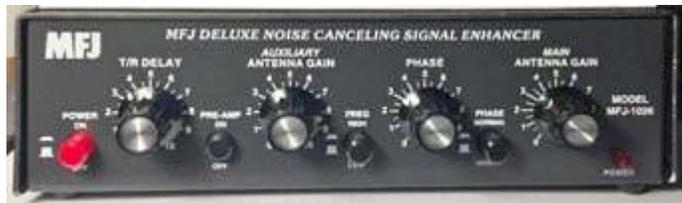
Close-up of MFJ-1026 Noise Canceling Signal Enhancer. Rotary controls are: T/R Delay, Auxiliary Antenna Gain, Phase and Main Antenna Gain. [N2MUZ pic]
