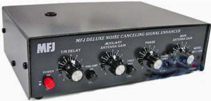
The MFJ-1026 Deluxe Noise Canceling Signal Enhancer. Hole in the cover is for a telescopic auxiliary antenna.
