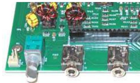
*Items normally emerging through the  $\mu$ BITX v6 front panel are (L to R) on/off-volume control, 3.5 mm microphone socket and 3.5 mm headphone socket.*
