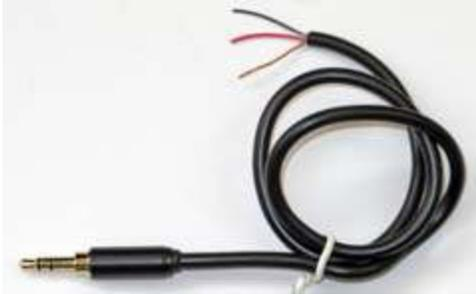
3.5 mm to 3.5 mm audio cable was cut in half, revealing shield conductor (sleeve), red wire (ring) and black wire (tip).
