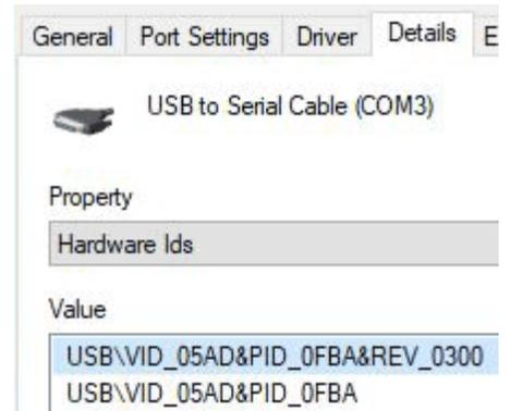
*Device Manager “Details” tab shows the Vendor ID and Product ID codes of a connected USB device in hexadecimal.*
