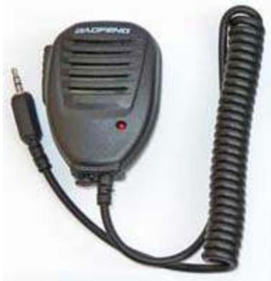
*Baofeng press-to-talk microphone as supplied by ‘HF Signals’ with the  $\mu$ BITX v6 kit.*
