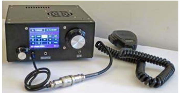
$\mu$ BITX v6 with Uniden BC645 replacement CB microphone plugged into MIC socket using the adapter cable.
