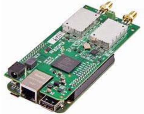
KiwiSDR is a software-defined radio (SDR) covering 10 kHz to 30 MHz, used at remote monitoring sites.
