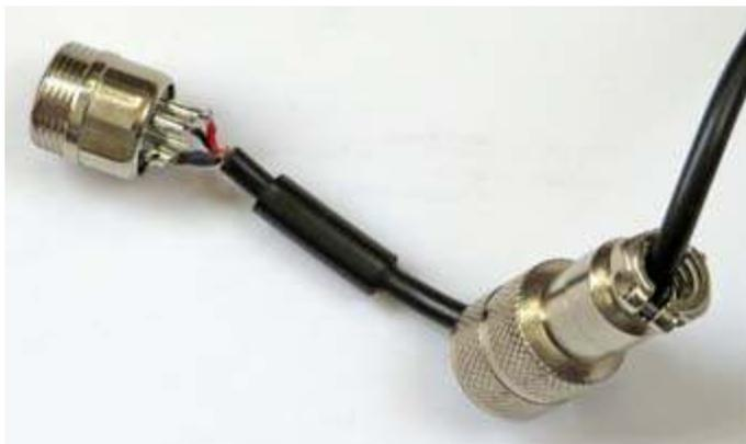
Wiring of the inline male “Foster 4-pin” connector. Note the vinyl tape building up the cable’s outside diameter to match the adapter’s cable clamp.
