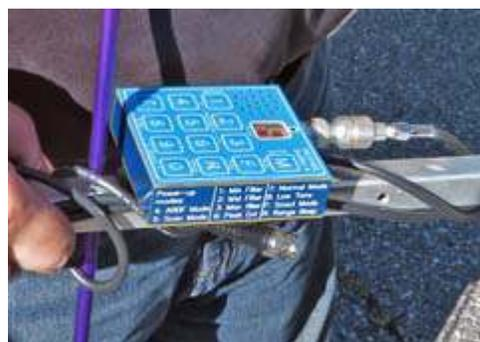
VK3YNG synthesized Foxhunt receiver mounted on boom of N2DVQ's antenna.
