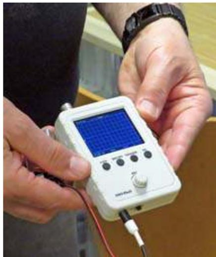
*Pocket-sized DSO Shell oscilloscope runs off a 9 volt battery.*
