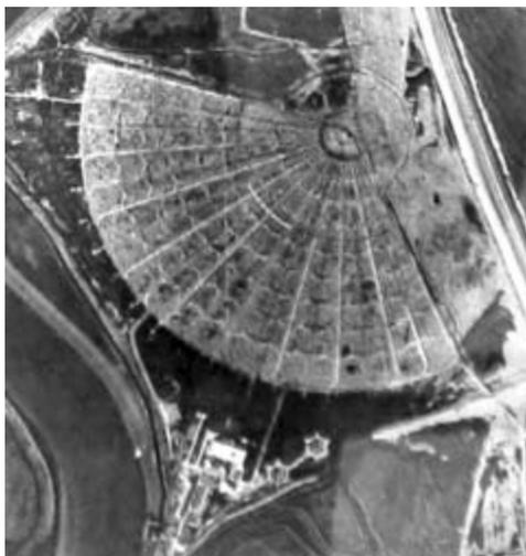
*Aerial view of 'Cobra Mist' antenna array at Orfordness. River Ore is lower left, North Sea is upper right. The site was subsequently used for BBC transmissions to Europe on 648/1296 kHz.*
