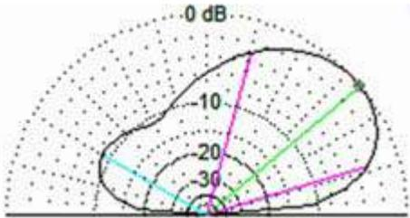
*EZNEC+ elevation plot for 2-element beam on 7.15 MHz calculated by NE2Q. Max gain 7.7 dBi at 40° elevation.*
