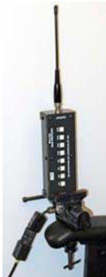
MFJ-762 as support for testing dual-band HT antennas. (Keep attenuation at 0dB to avoid damage.)
