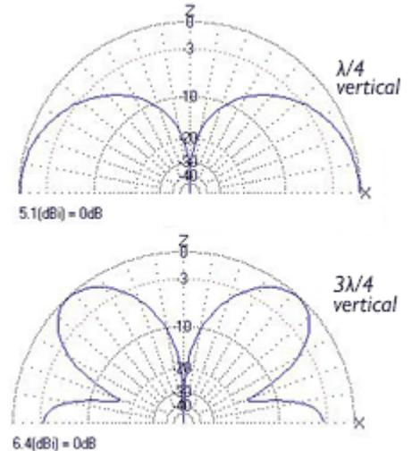
Elevation plots for  $\frac{1}{4}$ -wave vertical antenna (top) and same antenna used at  $3\times$  frequency — where it becomes a  $\frac{3}{4}$ -wave (below). Note the high-angle radiation from the  $\frac{3}{4}$ -wave. Software for plots: MMANA-GAL.
