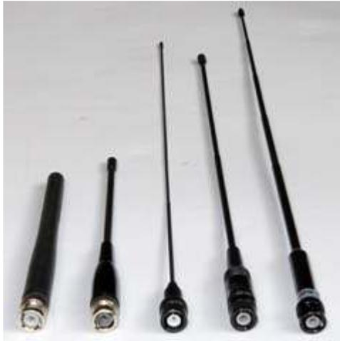
Flexible antennas with BNC connectors included in the test. L to R: BC125AT duck, Icom IC-W32 stock, Comet BNC24, Diamond RH77CA and MFJ-1712.
