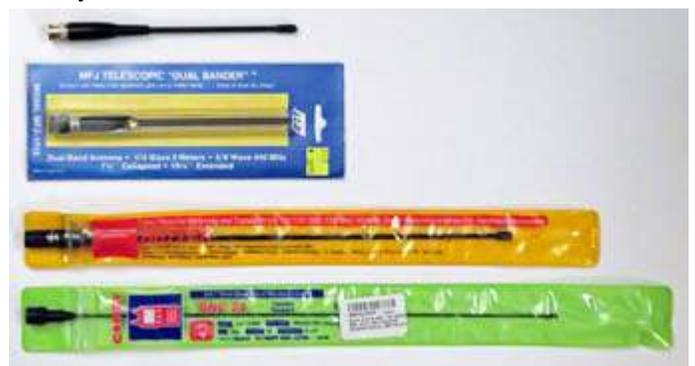
Best dual-band HT antennas of 2018. Top to bottom: Icom stock whip, MFJ-1712 telescopic, Diamond RH77CA and Comet BNC 24. SMA versions are also available.
