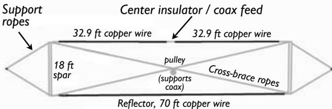
*N2CN 40 meter Yagi. Driven element and 70 foot reflector are spaced 18 feet apart and supported by two spars.*
