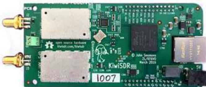
The KiwiSDR is a software defined radio receiver covering 10 kHz to 30 MHz. The unit is installed on a Beagle Bone single board computer connected to your LAN via Ethernet. The built-in web interface (OpenWebRX) can then provide browser access for 1-4 users.
