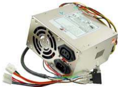
AT-style power supply has two Molex 6-way connectors for the motherboard.
