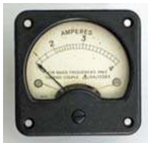
Radio-frequency ammeter with thermocouple movement from 1944. Note the non-linear scale.
