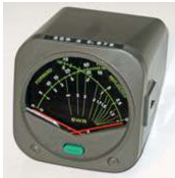
Daiwa CN-465M is a cross-needle power meter for the 144 and 440 MHz bands.
