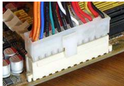
ATX 24-pin power supply connector plugged into a computer motherboard.
