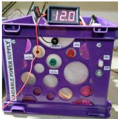
Testing output of the multi-voltage power supply between the yellow (+12V) and black (0V, ground) banana jacks.
