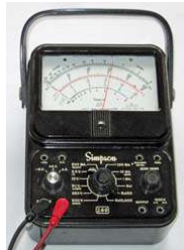
Simpson 260 series 6 analog VOM multimeter. The 260-8 is still manufactured today.
