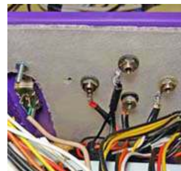
Power-on switch (left) and (right) four banana jacks are mounted on the insulated board. [N2CKD pics.]
