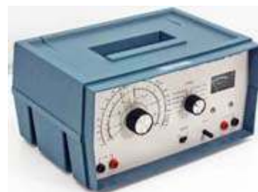
Heathkit IB-5281 RLC bridge can check the value of resistors, inductors and capacitors.
