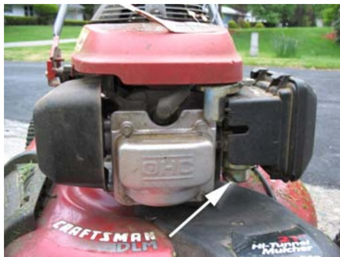
A blocked carburetor (arrowed) on this particular Honda engine helped inspire the article.
