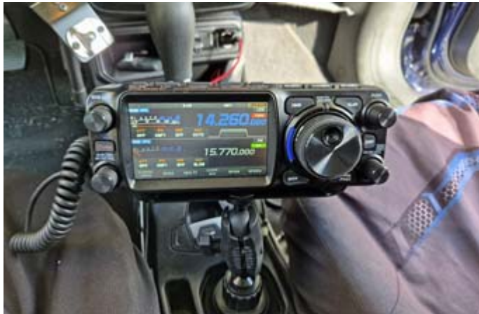
Yaesu "FTX-1optima" field head unit supported on a Lido ball-and socket cup-holder mount. [W2CH pics.]
