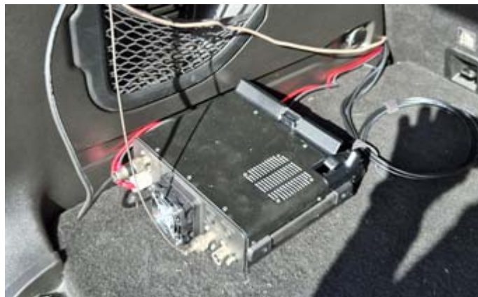
Yaesu FTX-1optima’s SPA-1 amplifier mounted in the trunk. [W2CH pics.]
