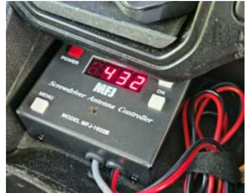
Ray's MFJ-1922B screwdriver antenna controller allows exact retuning of the adjustable HF antenna.
