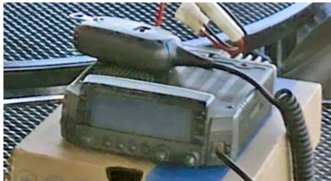
Kenwood TM-V7A dual-band mobile transceiver for 144 / 440 MHz as seen at April 18 PCARA Breakfast, Uncle Giuseppe's.
