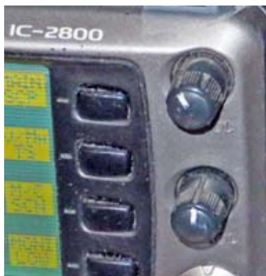
Volume and squelch controls on IC-2800 filled with white paint.
