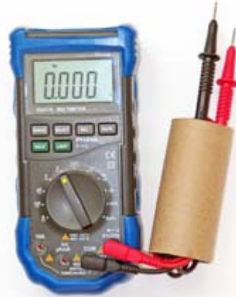
Wrap up test leads in the cardboard tube from a roll of bathroom tissue
