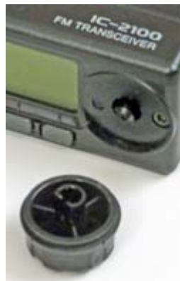
Push-on tuning dial knob (VFO/memory) for Icom IC-2100 2 meter transceiver.
