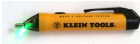
Klein Tools non-contact voltage tester indicates the presence of AC voltage with a red light. Green light shows that the internal AAA batteries are operational.
