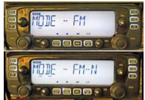
Menu setting for Icom IC-2730 transceiver allows Operating Mode choices of “FM” ( \pm 5 kHz max deviation) or “FM-N” ( \pm 2.5 kHz max deviation).
