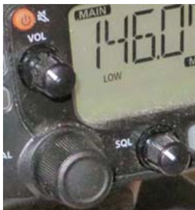
Volume and squelch controls on Icom IC-2730 marked with short strips of white vinyl tape.
