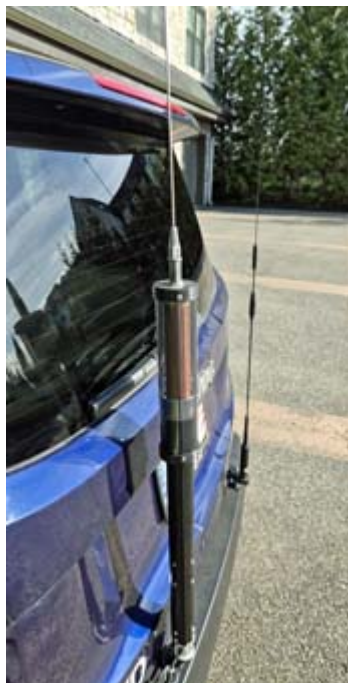
Antennas mounted on Jeep Renegade hatch are (left) Tarheel Little Pro and (right) Diamond CR320A. [W2CH pic.]
