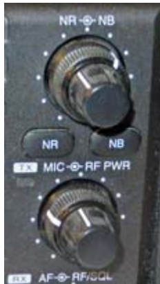
Control knobs on IC-7410 have a white paint stripe to indicate position.
