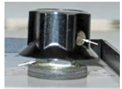
‘Antenna Matching’ control of MFJ-948. The arrowed 3/8” mounting hardware and Allen hex screw are all ‘hot’ to RF.
