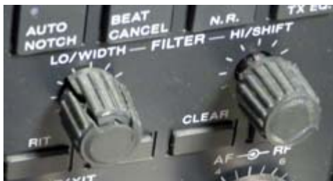
Cracked push-on control knobs on Kenwood TS-870 HF transceiver.
