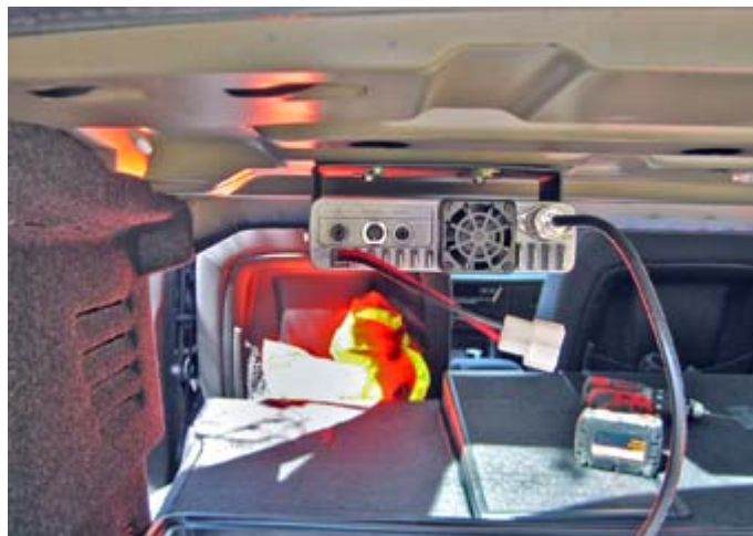
Icom ID-880H transceiver body mounted in the mobile bracket. [KD2EVI pic.]
