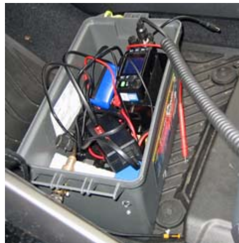
Go-Box on floor with TYT TH-6800 25 watt dual-band transceiver and Bioenno 4.5 Ah lithium iron phosphate (LiFePO 4 ) battery. [KD2EVI pic.]
