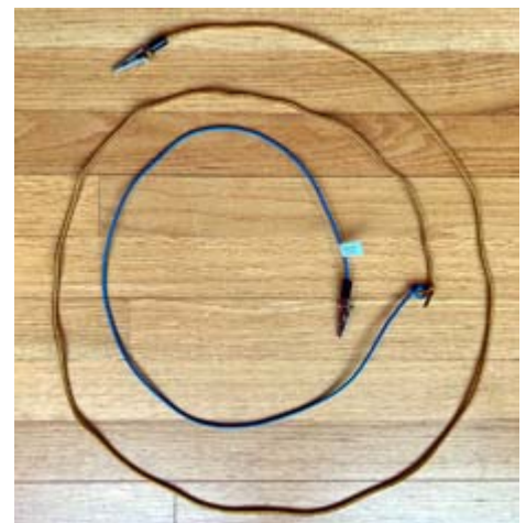
Karl connected 32" of blue wire to an alligator clip. The other end was extended with a shoelace. [N2KZ pics.]
