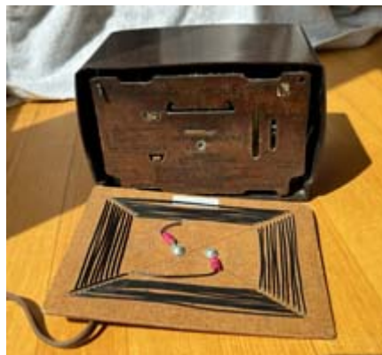
Spiral loop of wire wound on insulating board couples an external wire antenna to built-in antenna of a Motorola vacuum tube radio. [N2KZ pic.]
