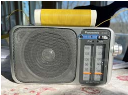
Coupling an external wire antenna to a portable AM radio using a coil of wire wound on PVC pipe. [N2KZ pic.]
