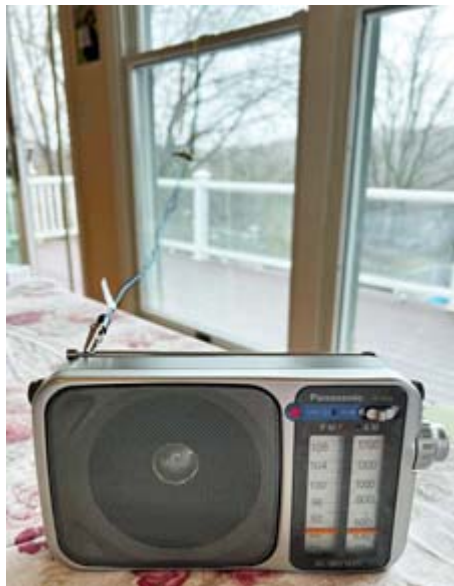
32" of wire connected to RF-2400 receiver's telescopic antenna by alligator clip and supported by shoelace attached to a window lock. [N2KZ pic.]
