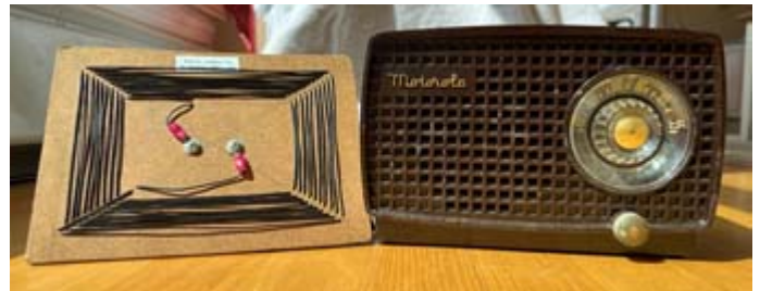
Move your loop closer or further away from the radio for the right amount of coupling. The radio here is a Motorola 59B11. [N2KZ pic.]
