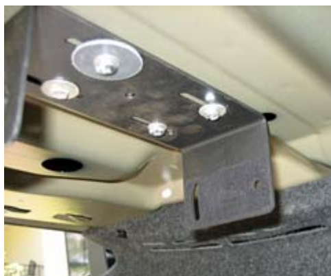
Mobile bracket installed under the rear package shelf. [KD2EVI pic.]
