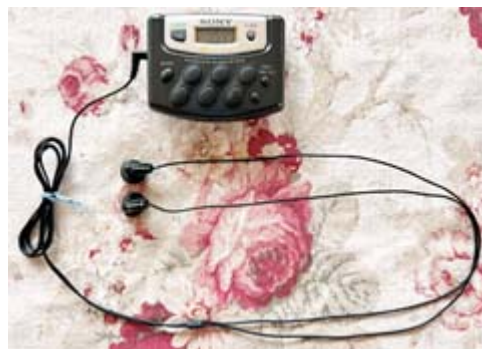
Folding the earbud cable back on itself may reduce signal overload. [N2KZ pic.]
