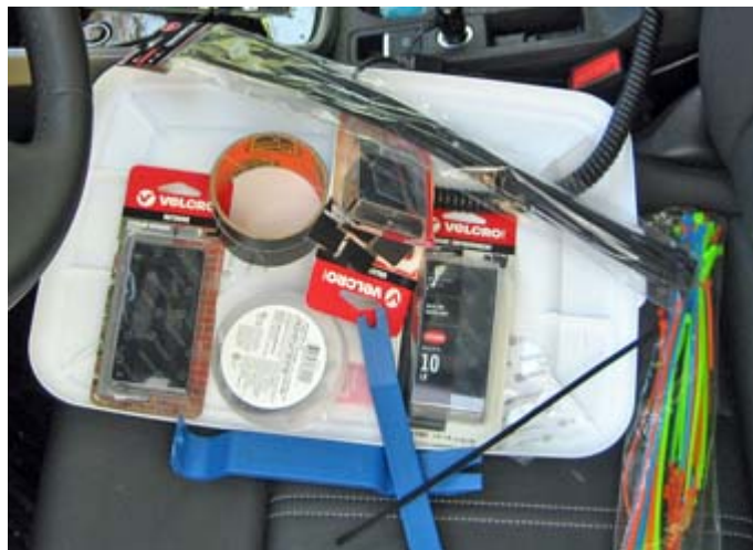
Plastic trim removal tools, Velcro, adhesive tape, zip-ties and other supplies used to install the ID-880H. [KD2EVI pic.]
