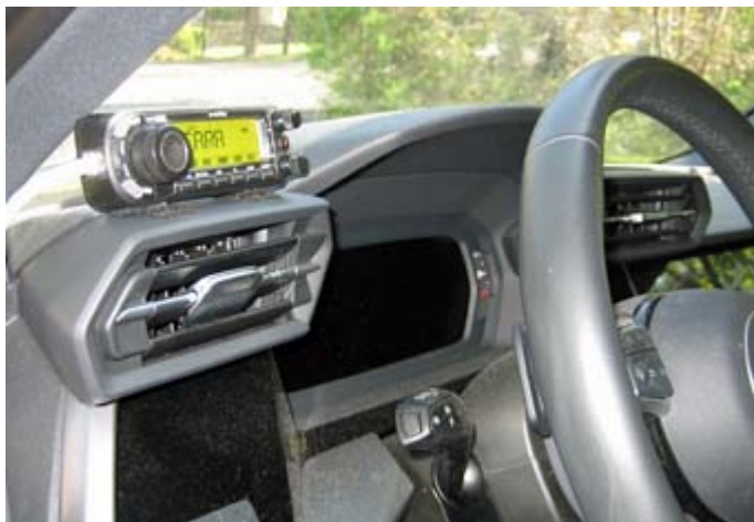
ID-880H control head secured to the Audi dashboard using Velcro sticky-back squares. [KD2EVI pic.]
