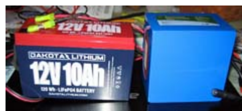
10 Ah Dakota Lithium battery (left) and 12 Ah Bioenno Power LiFePO 4 battery.
