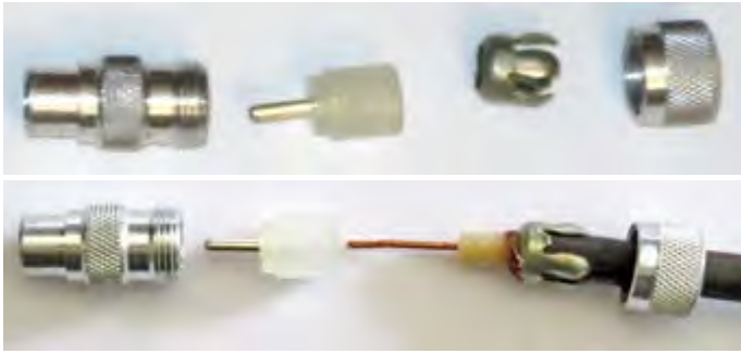
Top: Belling-Lee L734/P/AL polished aluminum coaxial plug disassembled. Below: Low-loss TV coaxial cable cut to length ready for soldering inner conductor to L734 center pin. Collet clamp grips cable and traps outer braid.
