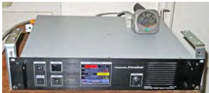
PCARA's Yaesu DR-1X System Fusion repeater being reconfigured for use on 146.67 MHz in September 2022.
