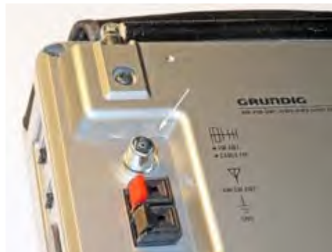
Grundig S350 AM-FM-SW receiver has a Belling-Lee style antenna socket (arrowed) for the FM antenna connection.
