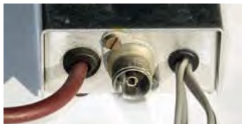
Home-built attenuator incorporated a Belling-Lee 75 ohm coaxial socket mounted on the aluminum chassis.
