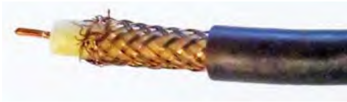
Low-loss 75 ohm TV coax from the U.K. with solid copper inner conductor, foamed polyethylene dielectric, braided copper outer conductor and flexible PVC sheath.
