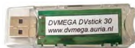
DVMEGA's DVstick 30 lets you make a digital voice QSO without a radio. All you need is a Windows PC with sound card, microphone, speaker and the BlueDV software. [DVMEGA.]
