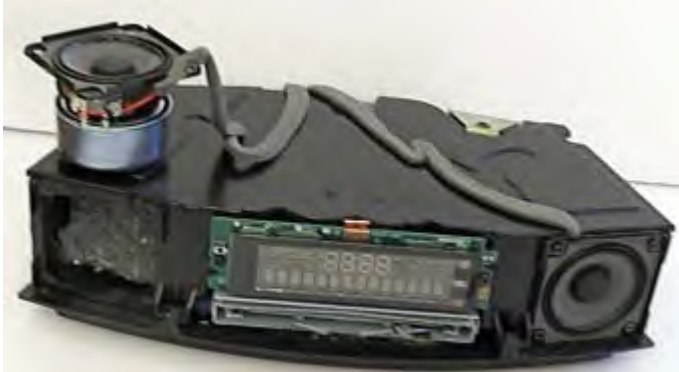
Bose Wave Radio with top cover taken off and left-hand acoustic driver unit unscrewed then lifted out.
