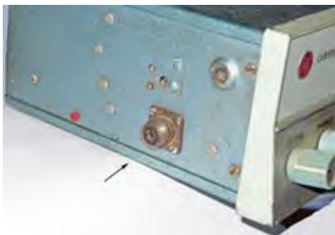
Pye Cambridge VHF mobile radiotelephone with Amphenol SO-239 antenna socket (arrowed) on the left side. Surplus Pye equipment was popular with U.K. radio amateurs in the 1970s.
