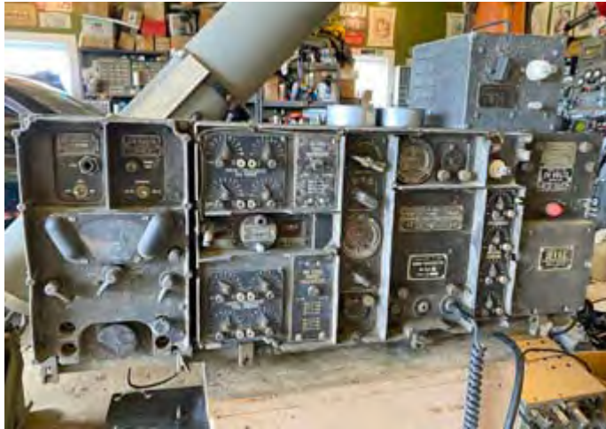
Old equipment – BC-652 receiver and BC-653 transmitter.
