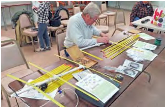
David K2WPM assembles a tape measure Yagi antenna from its component parts.
