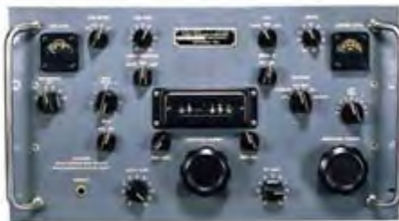
R-390 communications receiver covered 0.5 - 32 MHz and weighs 65 lb.
