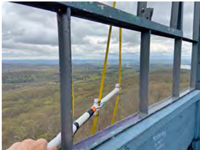
David K2WPM points his new tape-measure Yagi antenna from Mt. Ninham fire tower. [K2WPM pic.]
