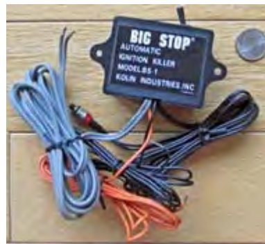
'Big Stop' vehicle immobilizer automatically interrupted ignition circuit. Installation could save up to 15% on insurance. [NE2Q pic.]
