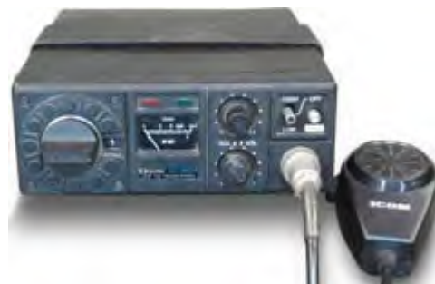
Icom IC-22A was an all solid-state 2 meter FM transceiver with 22 crystal-controlled channels.
