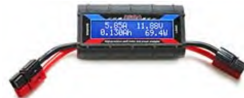
Inline meter with Powerpoles displays voltage and current.
