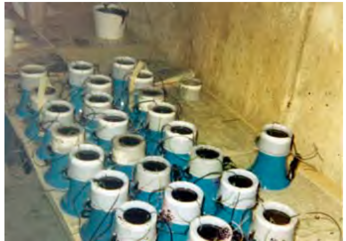
Early siren production in the basement of Jay's father's home in Lake Mohegan, 1970. Electronic circuitry was potted in epoxy behind the speaker horn. [NE2Q pic.]
