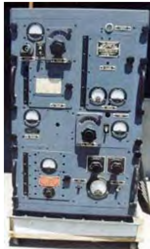
1946 YG-1 radio homing beacon produces 25 watts on 246 MHz, feeding Morse Code letter bearings to a rotating antenna.
