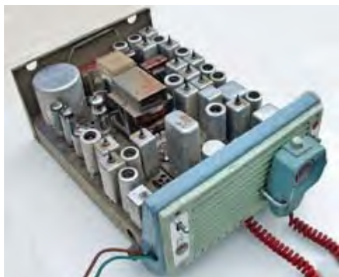
Pye Ranger mobile transceiver had a total of 19 vacuum tubes.
