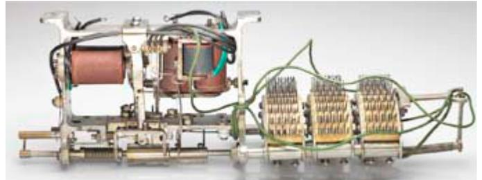
*Strowger step-by-step two-motion exchange selector, 1898.*
