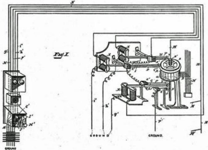
*A.B. Strowger’s U.S. Patent 447,918 of 1891 showed telephone equipment at left with telegraph keys G, H and I activating electromagnets in the Exchange to move a contact vertically then horizontally around a cylinder.*
