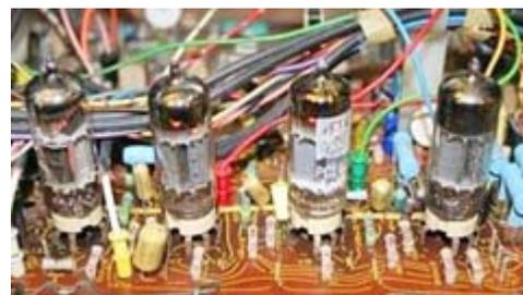
*Pye color television from the early 1970s had hybrid circuitry with three PCL84 tubes for color difference outputs. (TV sweep tubes like the PL509 and 6HF5 were used in amateur radio HF amplifiers.)*
