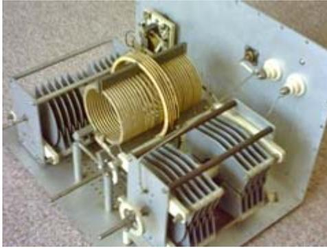
View inside a Johnson Kilowatt Matchbox tuner for balanced lines. Note the size of the matching components.
