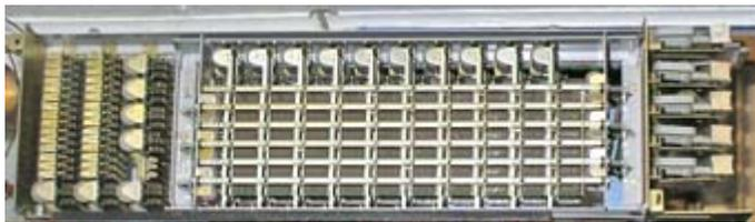
*Crossbar switch has horizontal and vertical bars activated by electromagnets.*
