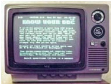
*NEC UHF-only “IC/Transistor” color TV from 1981 was all solid state apart from the CRT.*
