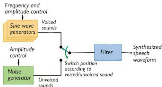
Decoder section of a voice encoder-decoder. [After Electronics Coach.]
