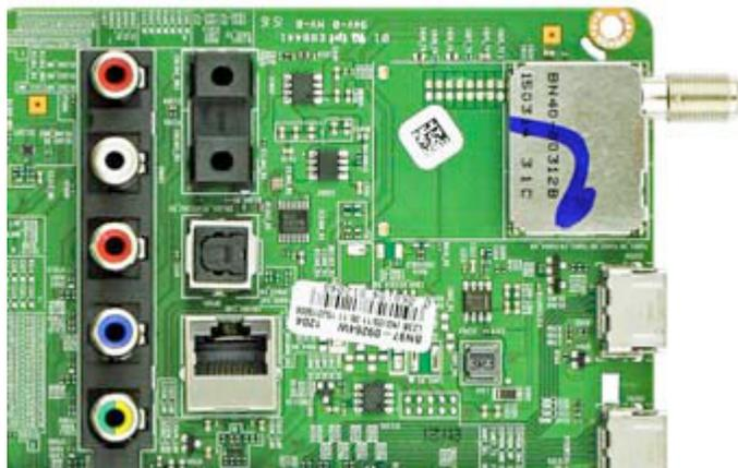
*Part of the main circuit board from a Samsung 55 inch LCD color TV shows over 100 surface mount devices. Component density increased and reliability improved with the change from wire-ended devices to SMD.*
