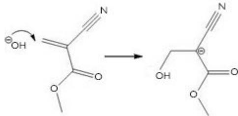
*Initiation step — a negative hydroxyl ion  $\text{OH}^-$  attacks the  $\text{C}=\text{C}$  double bond of a cyanoacrylate monomer.*
