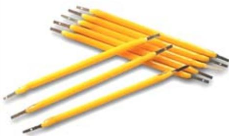
*These LED ‘filaments’ from Handsontec are each rated 1 watt, with a forward voltage of 70 - 80V DC, and a current of 13mA.*
