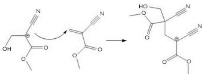
*Propagation step — anion formed in the initiation step attacks another cyanoacrylate monomer at the  $\text{C}=\text{C}$  double-bond. [After Univ of Bristol Molecule of the Month.]*
