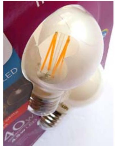
*Philips frosted glass globe lamp after the glass envelope was accidentally broken, reveals four LED filaments inside.*
