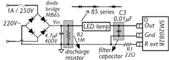
Application circuit from the SM2082B data sheet for measurement of RF interference level.
