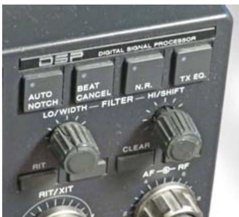
*LO and HI filter control knobs on the Kenwood TS-870 transceiver.*
