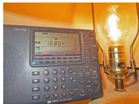
*Using a portable LW/MW/SW AM/FM portable radio to monitor RF interference from a GEC LED lamp. (No RFI detected.)*
