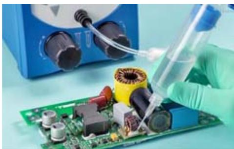
*Nordson dispensing equipment applies cyanoacrylate adhesive to an electronic assembly.*
