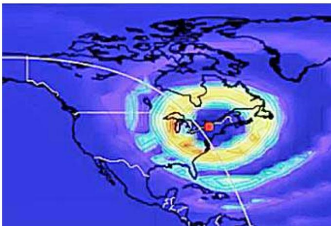
Propagation pattern for a normal HF antenna, optimized for low-angle radiation, leaves a **skip zone**, not reached by any sky wave.
