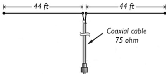
Simple half-wave dipole for 60 meters, 5.3 - 5.4 MHz.
