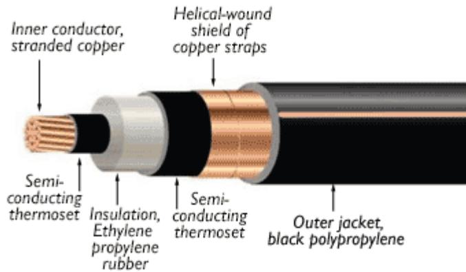
*Cutaway diagram of a medium voltage shielded cable. Three of these cables are twisted together for three-phase power distribution.*
