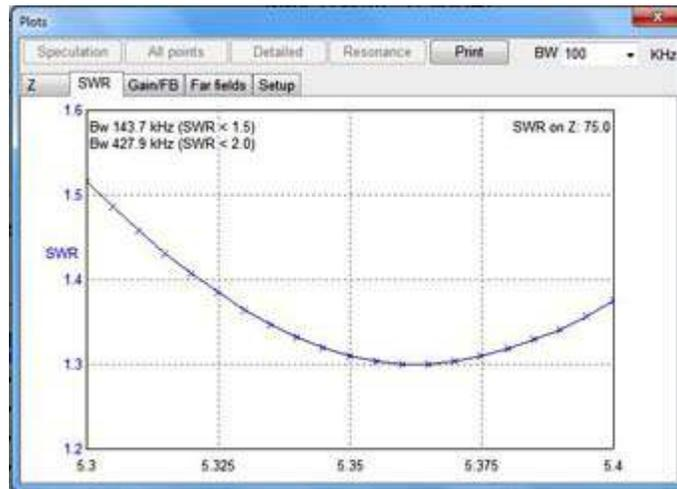
SWR predicted by MMANA-GAL software for a dipole 87.6 ft long, 33 feet above ground, resonant at 5.36 MHz.
