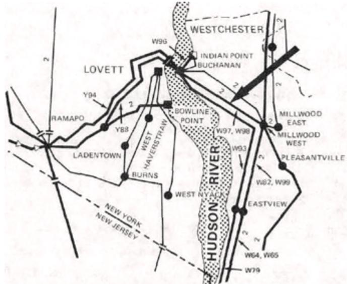
High voltage lines as described in DOE report "The Con Edison Power Failure of July 13 and 14, 1977". Arrow shows where lightning struck the 345 kV lines from Buchanan to Millwood, initiating the outage.
