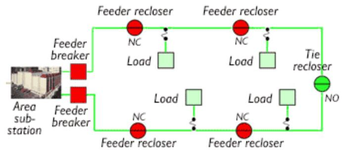
Con Edison overhead autoloop system for 4 kV, 13 kV and 27 kV feeders. NC = normally closed, NO = normally open. [After Con Ed presentation.]
