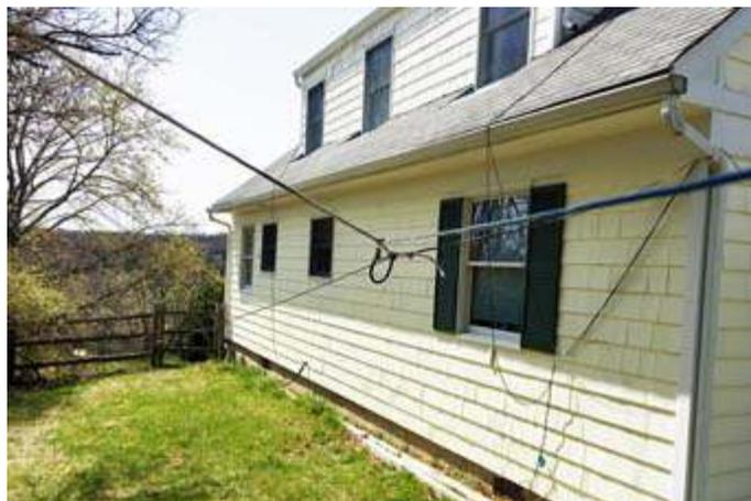
*New NVIS antenna for 5.3 MHz at Karl's location.*
