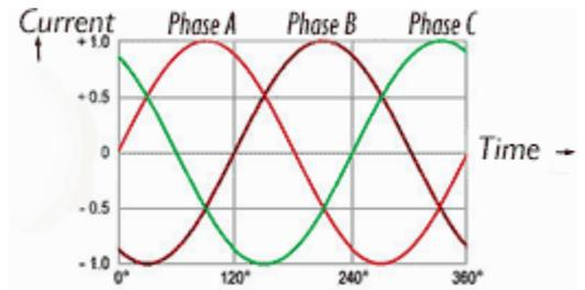
*Three phase alternating current. If the voltage between one phase and neutral is 120 V AC, then the voltage between any two phases is  $120 \times \sqrt{3} = 208$  V AC.*
