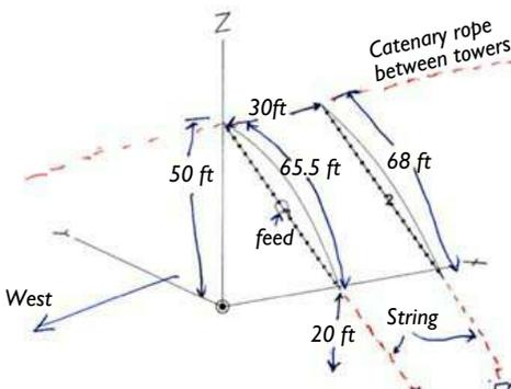
2-element sloping wire antenna for 40 meters designed by Jay, NE2Q.
