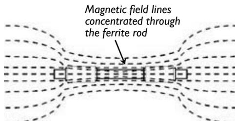
*In a loopstick antenna the ferrite material concentrates magnetic field through the wire coil(s), which have been wound around the ferrite rod.*
