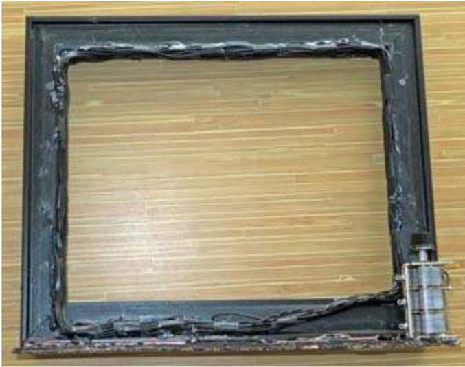
*View of Lovji's completed antenna with wire loop hot-melt glued to the photo frame and variable capacitor mounted lower right on the wooden base.*
