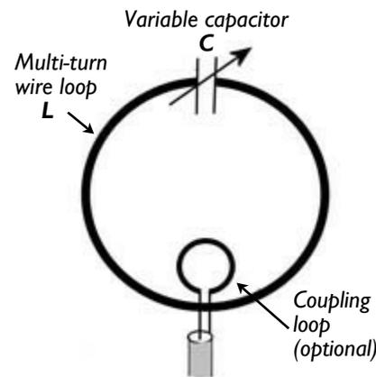
*Loop antenna consists of one or more turns of wire resonated with a variable capacitor.*
