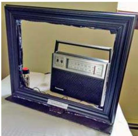
*Place the loop antenna near to a portable AM radio receiver. [N2CKD pic.]*
