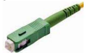
SC/APC green connector has 8° angled contact to prevent reflections traveling back down the fiber.
