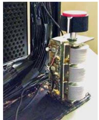
*Detail of MF loop antenna showing wire soldered to variable capacitor. [N2CKD pic.]*
