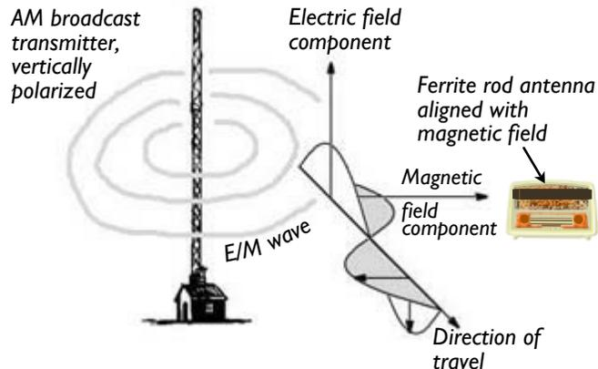
*Polarization of an electromagnetic wave is in the same direction as the **electric** field, which is vertical in the case of most AM broadcasts. Alignment of a receiver’s ferrite rod antenna for maximum signal should be in line with the **magnetic** field component — which is **horizontal** in this case and at right angles to the direction to the transmitter.*
