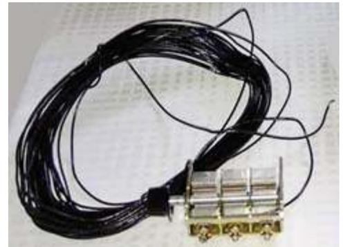
*50 feet of insulated wire and three-gang variable capacitor. [N2CKD pic.]*
