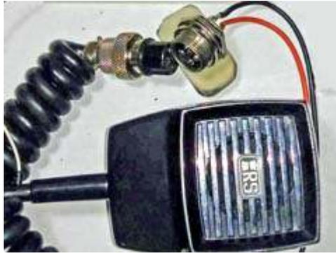
*Ex-CB dynamic microphone was wired through a 4-pin microphone socket to the three-transistor preamplifier.*
