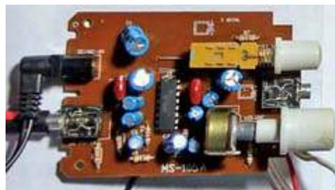
Circuit board from Lovji's computer speakers. Volume control is at lower right.
