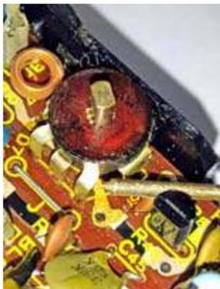
*Signal injector applied to radio's volume control.*
