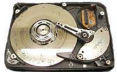
If the read/write heads of a hard disk drive hit the disk surface, then data is lost.
