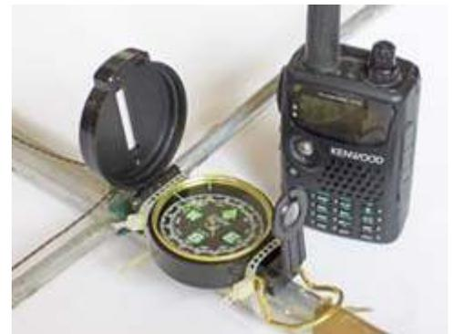
*Keep your compass away from magnetized objects such as an HT loudspeaker.*
