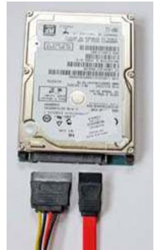
SATA hard drive with power cable (left) and SATA cable (right).
