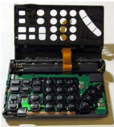
*Disassembling the lower section shows the ribbon cable threaded through the keyboard cover.*
