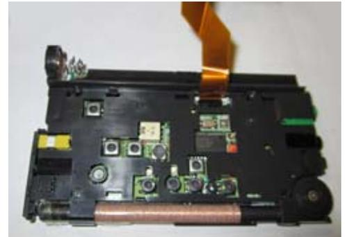
*Lower circuit board in the ICF-SW100 with ribbon cable attached.*
