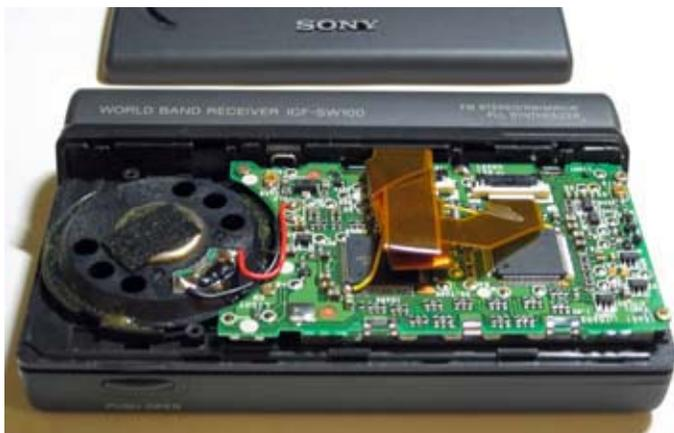
*Removing the top cover of the ICF-SW100, which is held on by plastic clips, reveals the loudspeaker, microprocessor board and two yellow ribbon cables.*
