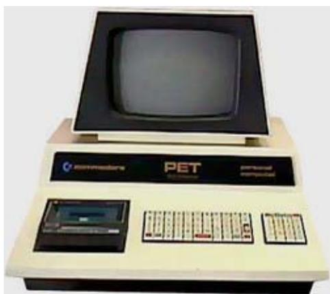
*Commodore PET was a self-contained microcomputer with cassette drive, keyboard and video monitor.*
