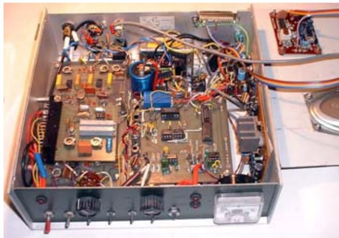
*G3VNQ RTTY/CW interface for the PET contained a Microtronics M-65 decoder as well as TU and AFSK boards from M.K. Products. This unit was subsequently modified to include RS-232 serial I/O for use with a PC.*
