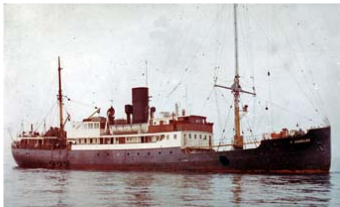
Radio Caroline North. Transmit antenna was a “vertical folded unipole 168 feet high” consisting of a wire cage attached to the top of the 155 ft mast. [CC BY-SA 4.0, Credit: DWSav.]
