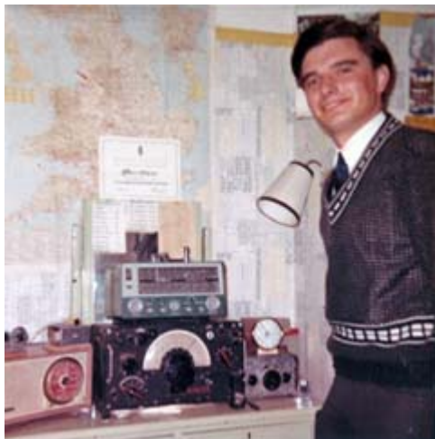
Southport radio room of six decades ago. R1155L receiver under Heathkit Mohican.
