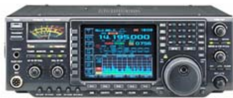
Icom IC-756Pro HF transceiver featured 32-bit IF-stage digital signal processing.
