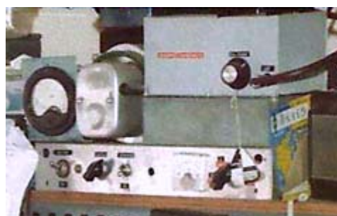
Home-brew amplifier for 144 MHz employed 4X250B and 1.2 kV DC supply.
