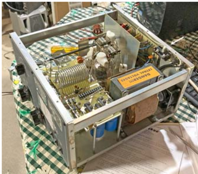
Joe's AL-811H amplifier with top cover removed. Note the orange warning label "DANGER!!! LETHAL VOLTAGES" and the safety interlock (arrowed) at rear of chassis.
