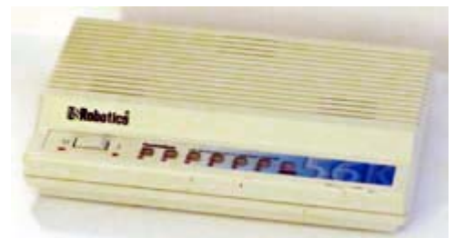
In April 2000, Internet connectivity required a dial-up modem connected to the phone line — like this USRobotics® V.90 56K model.
