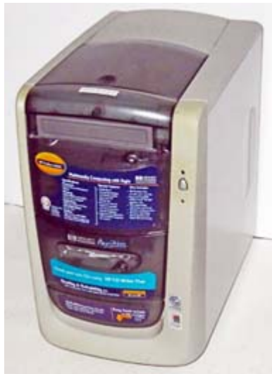
HP Pavilion 8595C with Pentium III, 128 MB RAM and 36 GB disk.
