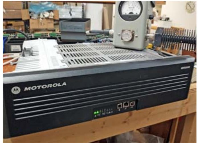
*The new Motorola MTR3000 repeater producing 50 watts output while on-test into dummy load. [N2CBH pic.]*
