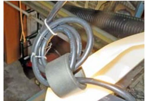
Door opener’s power cord looped three times through the ferrite toroid.
