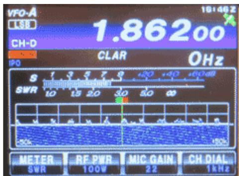
*Broadband interference caused by sparks from 60 Hz AC electrical equipment appears as spikes on the FT-991A scope display, apparently moving across the frequency spectrum, producing diagonal lines on the waterfall. [The source was an electric drill with sparking commutator].*
