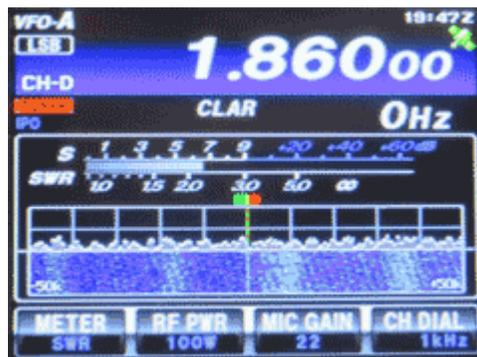
*Noise level experienced on 160 meters. Broad peaks at steady frequencies on the waterfall display suggest problems with a switch-mode power supply.*
