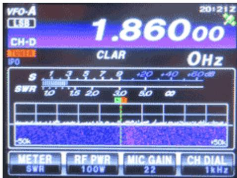
Noise level on 160 meters was back to the same S-meter reading as when the garage door opener was unplugged.
