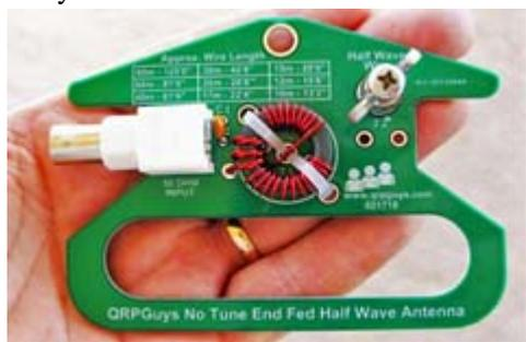
QRPGuys portable no-tune end-fed half wave antenna kit. (You provide the wire.)
