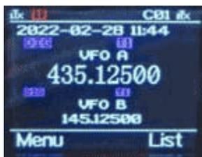
Standard display with VFO A on top, VFO B below (actual size).
