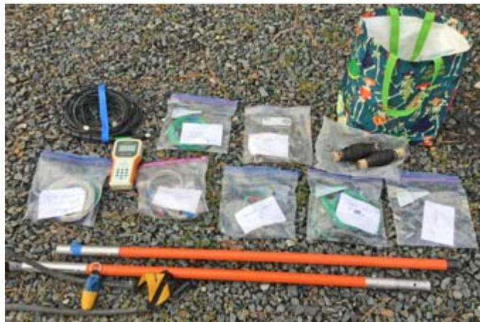
Coaxial cable, wire elements in baggies, cord and analyzer all fit into a shopping bag. Poles below are part of the Notch Big Shot antenna launcher. [K2WPM pic.] [Sling shots are legal in NY State provided they do **not** have a wrist brace. Check local regulations and use with caution. -Ed.]
