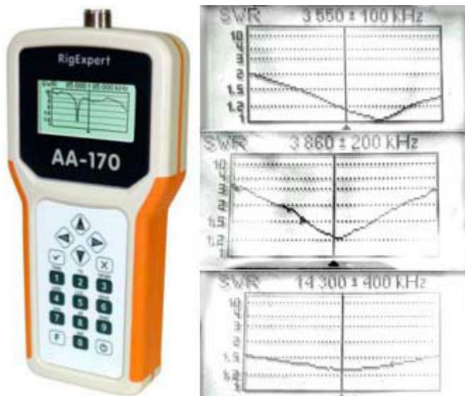
Graphs for K2WPM's inverted-V linked dipole antenna. Top, SWR is less than 2.0:1 across 200 kHz on 80 meters; middle, less than 3.0:1 for a 400 kHz bandwidth on 75 meters. Below, less than 1.5:1 over the whole 20 meter band.
