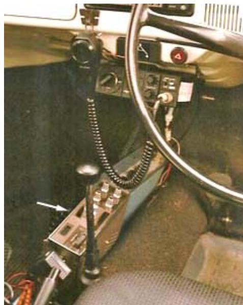
*Belcom Liner 2 (arrowed) was installed near the Beetle’s gear shifter alongside a Pye Westminster for 4 meter AM. Icom IC-22A is mounted above.*
