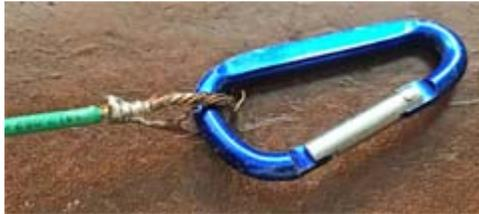
Original termination of each wire segment by snapping wire loop into a carabiner.
