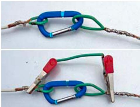
Carabiners insulated with shrink-wrap tubing. At top, insulated wire loops are snapped into an insulated carabiner. Below, wire segments are linked using a wire jumper with alligator clips. [K2WPM pics.]
