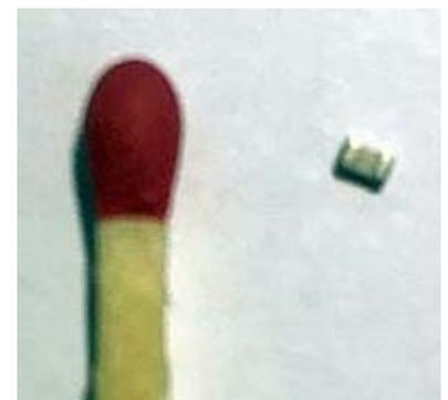
Surface mount capacitor, part of the LP1's low pass filter, shown against a match-head. [N2MUZ pic].
