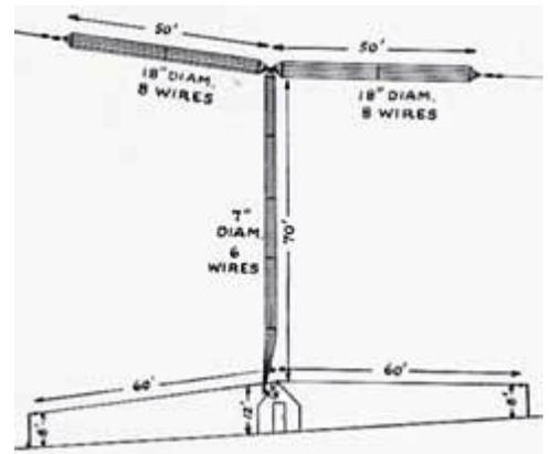
Antenna for Transatlantic Test station 1BCG, Greenwich was suspended between two masts — 108 ft and 75 ft high. Station hut is below the counterpoise.
