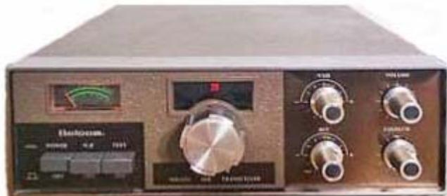
*Belcom Liner 2 144 MHz SSB transceiver. Push buttons at left for POWER, NB and TEST. Channel selector center. Controls at right for VXO, VOLUME, RIT, and SQUELCH.*
