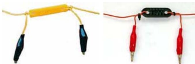
Two different plastic insulators with wire segments terminated in alligator clips for use in a linked dipole. The insulator at left is from SOTABeams.
