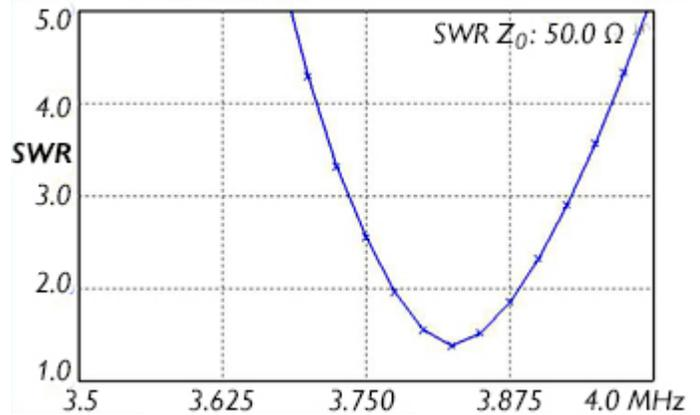
Limited bandwidth of an 80 meter wire dipole. A horizontal dipole cut for a frequency of 3.800 MHz has a bandwidth of 195 kHz for SWR < 3.0:1. [Prediction by MMANA-GAL software.]
