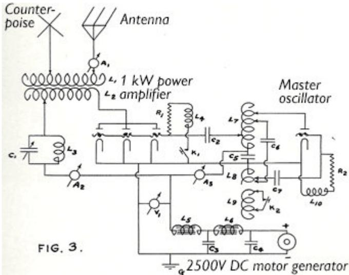
FIG. 3. Schematic of the 1kW CW transmitter at 1BCG for 1921 Transatlantic Test. RCA UV-204 triode in master oscillator drives three UV-204s in parallel in power amplifier.
