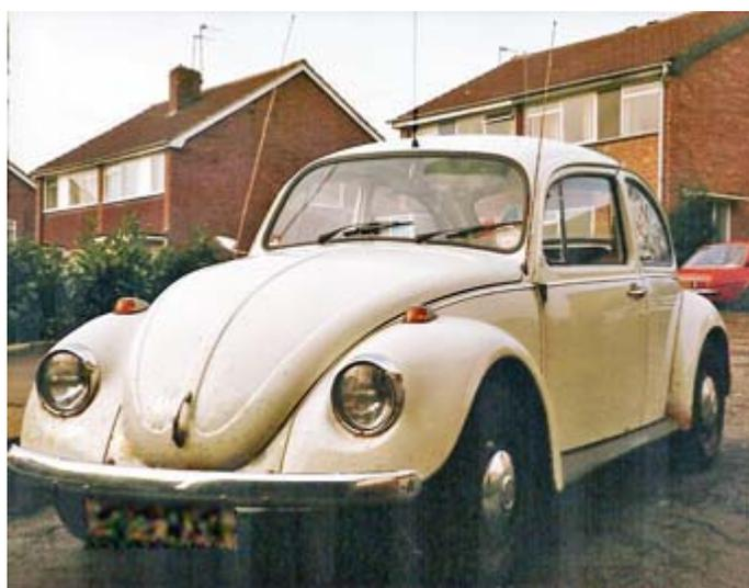
VW Beetle 1200 had antennas for (left) 4 meter AM, 2 meter FM (roof center) and 2 meter SSB (right).
