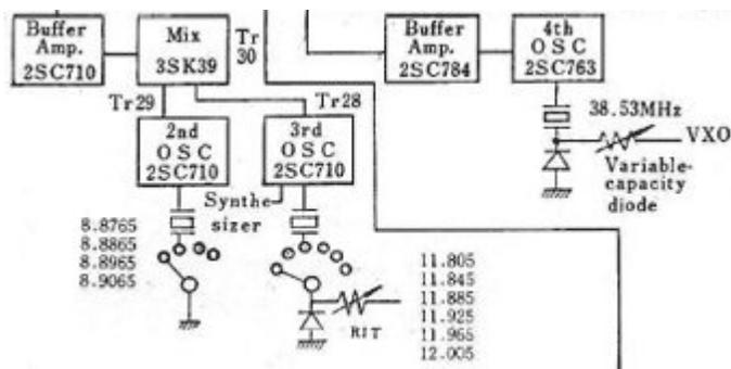
*Detail from Liner 2 block diagram showing the switched crystal synthesizer (2<sup>nd</sup>, 3<sup>rd</sup> OSC) and 4<sup>th</sup> crystal oscillator.*
