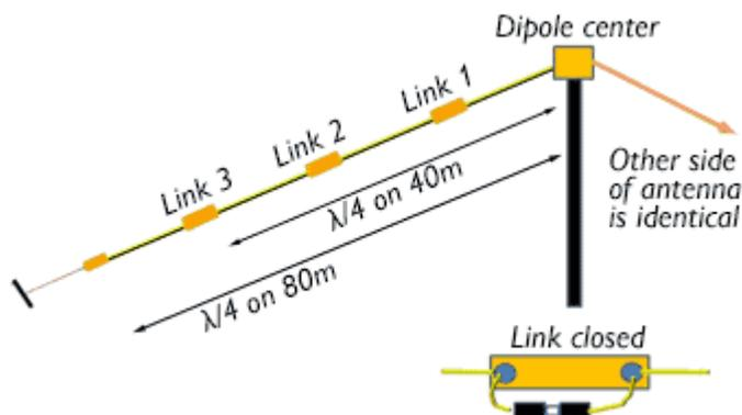
Linked dipole for four different HF bands in inverted-V configuration. Links are closed or opened to change bands. [After SOTABeams]
