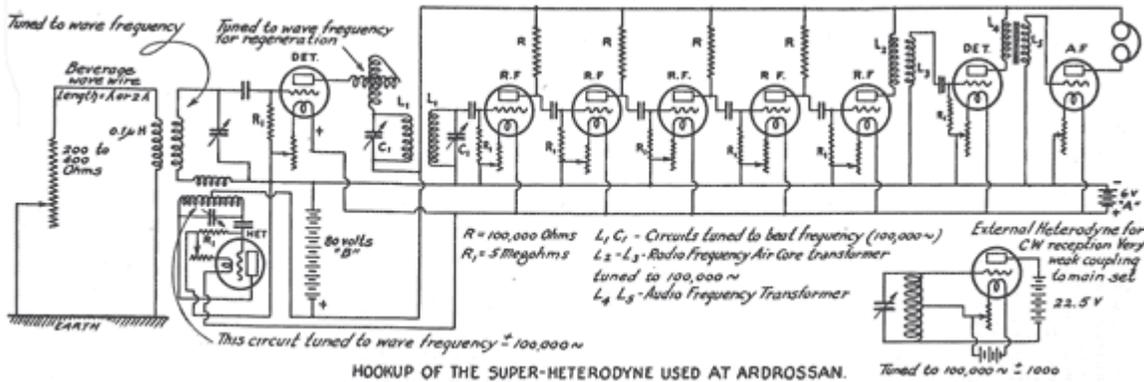
HOOKUP OF THE SUPER-HETERODYNE USED AT ARDROSSAN. Superheterodyne receiver used for Transatlantic Test by Paul Godley 2XE at Ardrossan, Scotland. Intermediate Frequency (IF) was 100 kHz. Local oscillator is at lower left, BFO at lower right.
