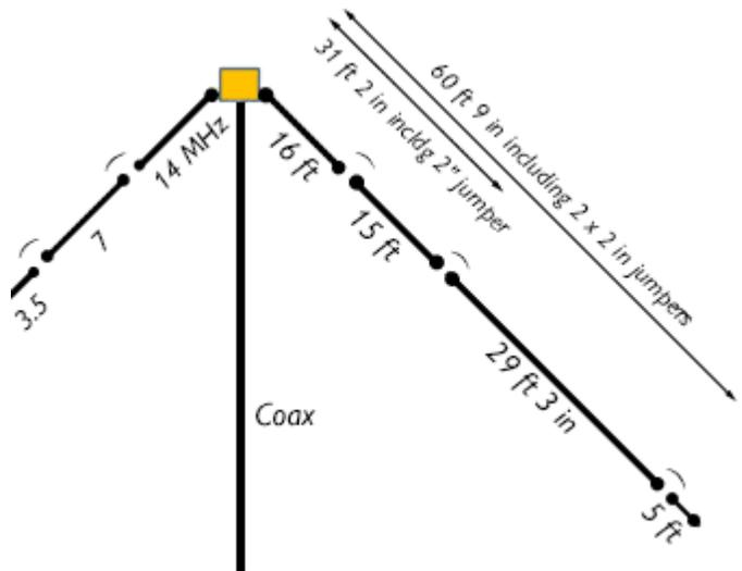
Diagram of one side of the linked inverted-V dipole as constructed by K2WPM. 5 ft segment at right is connected to extend the 75 meter / 3.85 MHz dipole for use in the 80 meter / 3.550 MHz CW section of the band.
