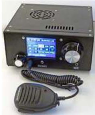
*$\mu$ BITX v6 seven-band QRP SSB/CW transceiver.*
