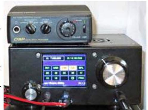
*Radio Shack DSP40 audio filter (top) is connected to the  $\mu$ BITX v6 audio output.*
