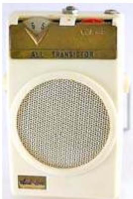
*Aud-Ion vintage two-transistor AM radio. [N2KZ pic.]*
