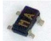
Sony SGM2016M dual gate GaAs MES FET — as used to repair the front end of a Yaesu FT-8000 transceiver.
