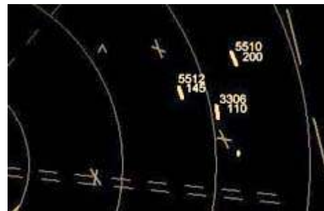
Radar screen showing transponder ‘squawk’ codes and aircraft heights (hundreds of feet).
