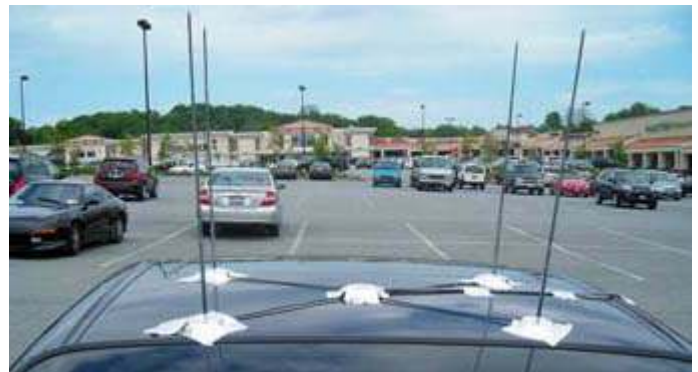
Ramsey Electronics Doppler DF antennas mounted on the roof of the KC2NKK/W2CH vehicle.
