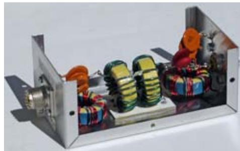
W3NJN bandpass filter for 40 meters (7 MHz) with the cover off. In order to protect adjacent amateur bands, this model has an insertion loss of 38dB at 4 MHz and 70dB at 14 MHz.
