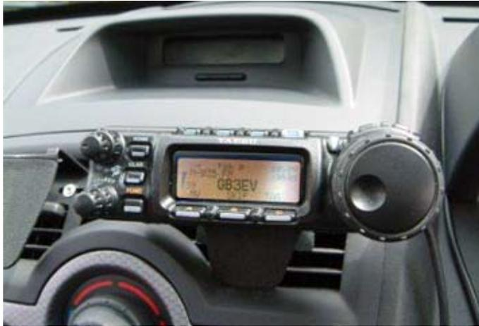
*W2CH has the control head for a multiband Yaesu FT-857D transceiver mounted on the dashboard.*
