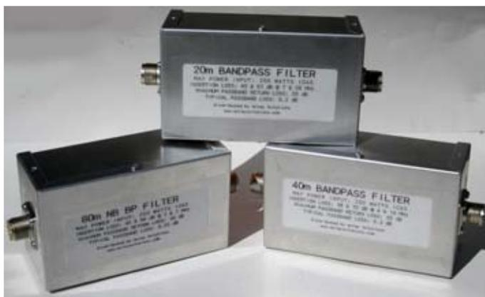
W3NJN bandpass filters for 80, 40 and 20 meters as used during PCARA Field Day.
