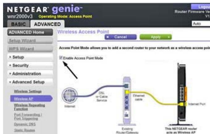
WNR2000v3 advanced menu allows simple setup as a Wireless Access Point through a single checkbox (arrowed).
