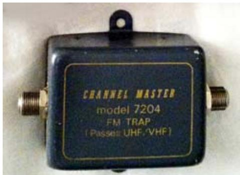
FM traps for 75 ohm TV feeder by Jerrold Electronics (top) and Channel Master.
