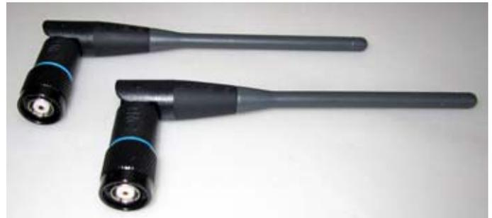
*Stock antennas supplied with the Linksys WAP54G have a reverse-polarity TNC plug connector.*
