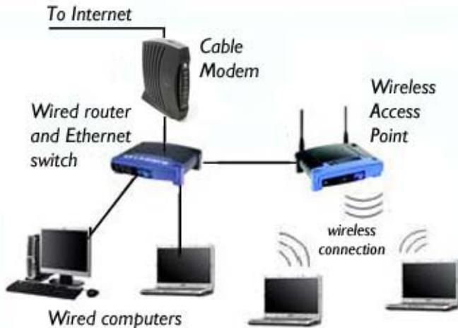
*Use of a separate Wireless Access Point with a wired Router/Ethernet switch can provide better wireless coverage.*
