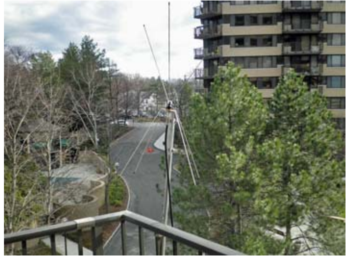
MP Super-M multiband antenna mounted on the balcony at the location of Ray, W2CH. [Photo by W2CH]
