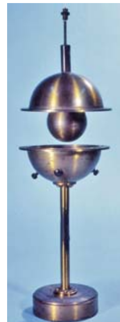
Faraday's apparatus for determining dielectric constant of insulators.
