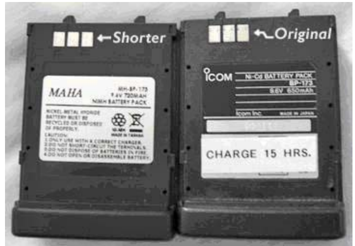
Maha NiMH replacement for the Icom BP-173 NiCd battery had shorter connection tabs than the original.
