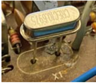
10.6975 MHz carrier oscillator crystal X1. [KA1HVR pic.]
