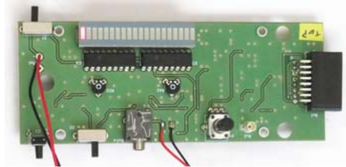
“Topside” of the main circuit board with all through-hole components inserted and soldered.
