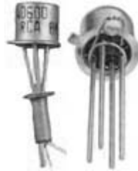
RCA 40600 dual-gate MOSFET with brass collar (left) or shorting spring.
