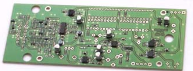
The ‘EMV-Spion 2.0’ kit has all the surface mount devices pre-installed on one side of the printed circuit board.
