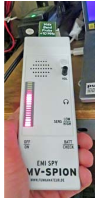
EMI Spy 2, with “Wide Band Probe < 10 MHz” inserted, detects noise from a switch-mode power supply.
