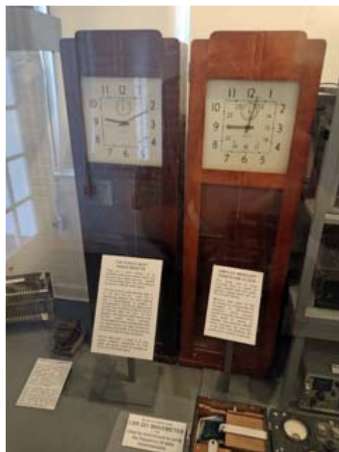
Seth Thomas mercury-compensated pendulum clocks used for timing 290 kHz radio beacon transmitters at Ponce Inlet Light. [Credit: KD2EVI]
