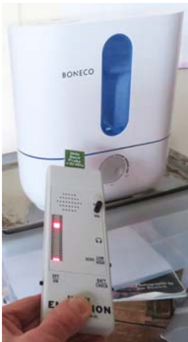
EMI Spy 2.0 found a strong signal from an ultrasonic humidifier.
