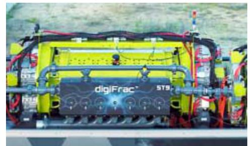
Liberty digiFrac pump has five electric motors on each side, each capable of 400 hp continuous or 550 hp peak.
