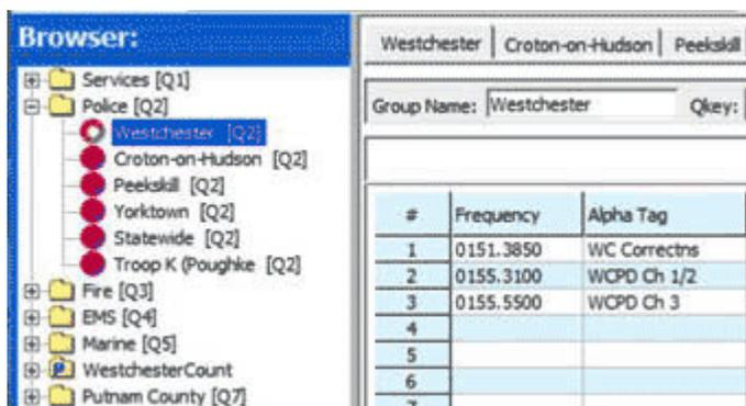
*Memory channels from Uniden BCT15X were transferred to the BCD996P2 scanner using Butel’s ARC-XT software. Each yellow folder is a “System”. Each red circle is a “Group”. Quick-keys are indicated by [Q1] [Q2] etc.*
