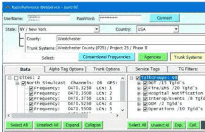
Importing details for Westchester County's P25 Phase 2 trunking system from RadioReference into ARC-XT.
