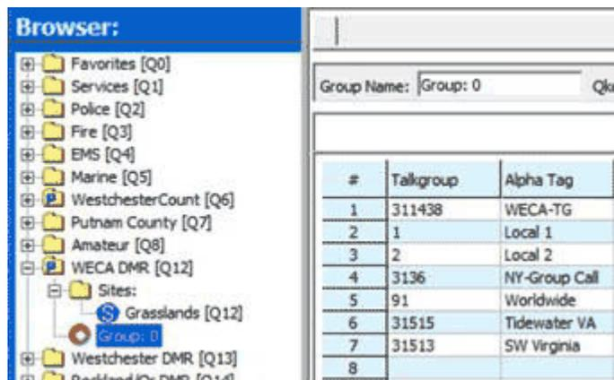
DMR repeater with multiple talkgroups is set up in Butel ARC-XT software as a system with type “DMR”. The ‘Site’ (blue ‘S’ lozenge) holds the frequency and color code. The ‘Group’ (red circle) contains talkgroups and time slots.
