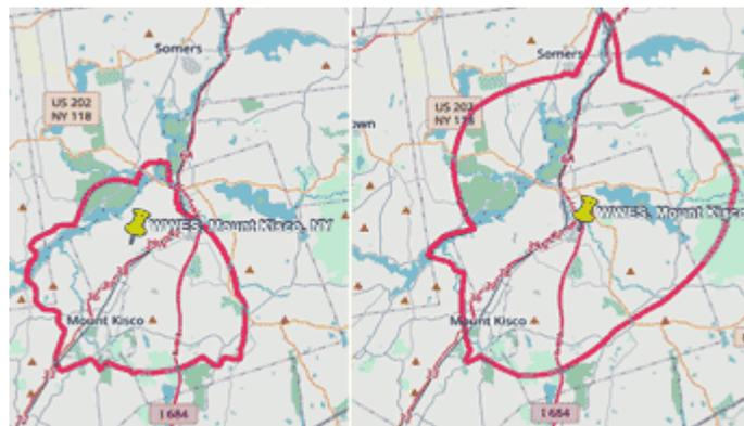
Transmitter coverage of WWES 88.9 MHz, Mount Kisco before (left) and after site move and power change.
