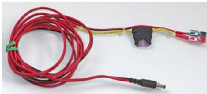
*12V DC power cable constructed with coaxial power plug included in the kit, inline fuse and Anderson Powerpoles.*
