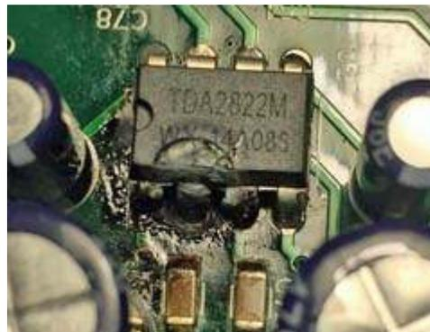
Todd's TDA2822M WX audio output IC which failed shortly after completion of the kit. [N2MUZ pic].
