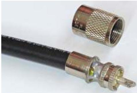
*Don't let this happen to you! Slide the shell/cover/coupling ring onto the cable before soldering.*
