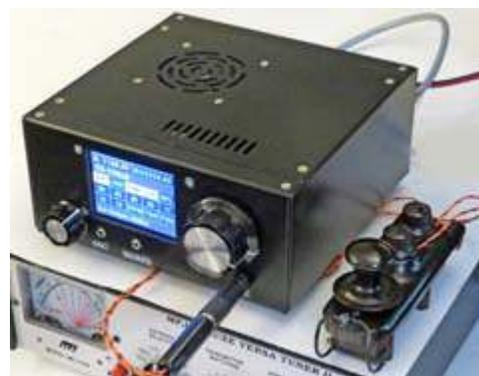
*$\mu$ BITX v6 set up for CW operation with a straight-key.*
