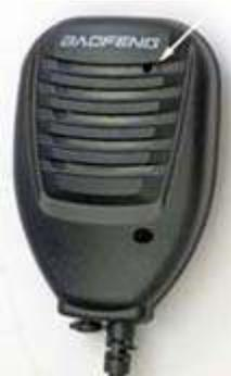
*Baofeng speaker/microphone with position of the electret element arrowed.*
