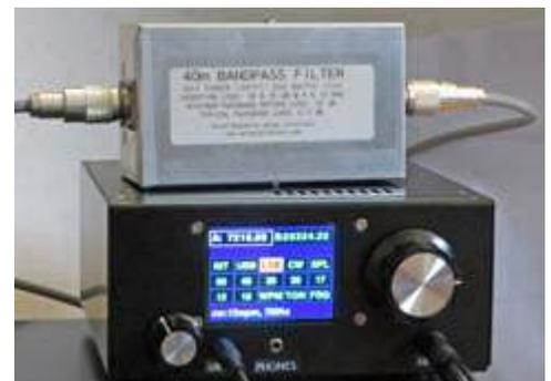
40 meter Bandpass Filter from Array Solutions stands atop the  $\mu$ BITX v6.
