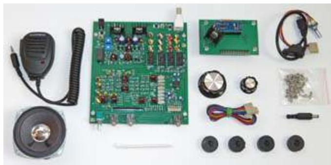
*Circuit boards and smaller components included in the  $\mu$ BITX v6 Full Kit.*
