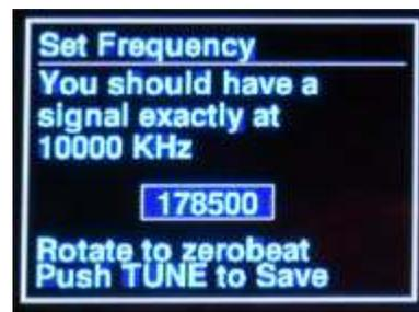
*Setting the  $\mu$ BITX v6 frequency for accurate tuning of WWV on exactly 10.000 MHz.*
