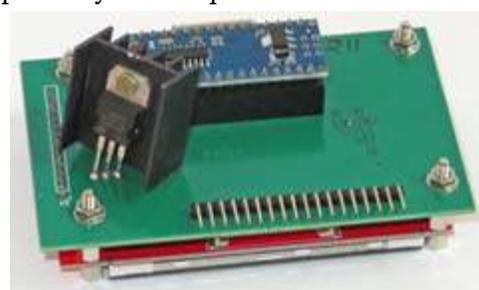
*Raduino assembly had the 7805 voltage regulator and heat sink twisted around.*
