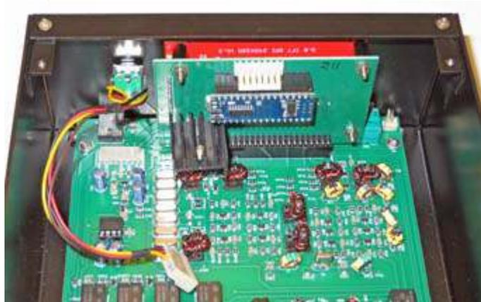
*Raduino assembly has been plugged into the main circuit board and fastened to the front panel. Rotary encoder cable (left) is ready to be connected to the Raduino.*
