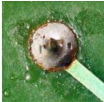
*Cold-soldered joint. Note the dull gray color of the solder.*
