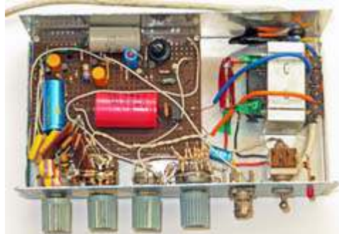
Inside the old audio signal generator.
