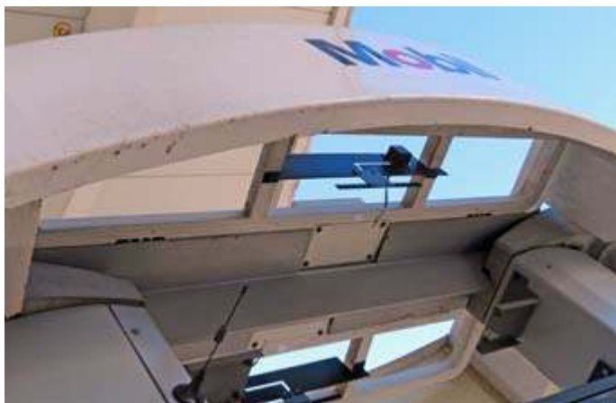
Looking up into the top of a Mobil gas pump reveals the molded plastic LF antennas for sending to the vehicle's transponder and slot antennas for UHF reception.
