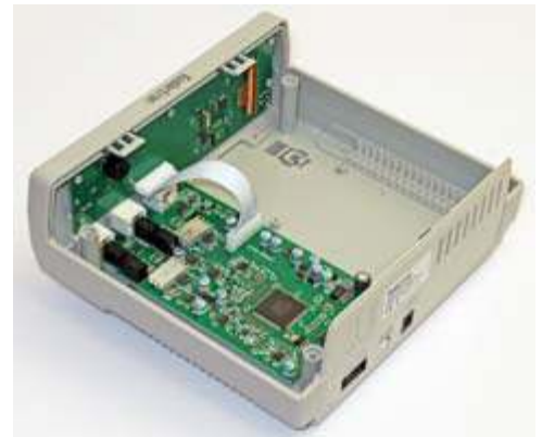
JDS6600 signal generator with top cover removed. The plastic case is not shielded.
