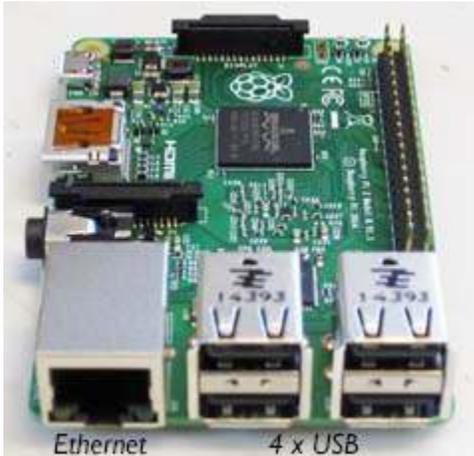
End-view of the Raspberry Pi 2 card shows the Ethernet port and four USB ports.
