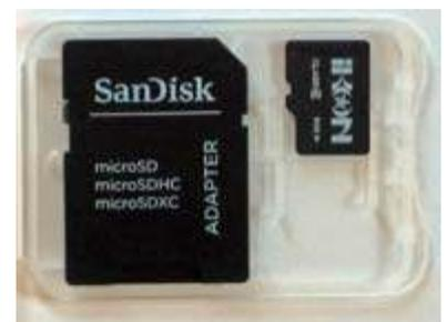
Raspberry Pi 2 storage employs 8GB-16GB microSD card (right). Adapter on left allows use in a standard SD card slot as used on many PCs.
