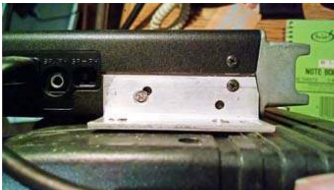
Close-up of the L-bracket that Bob used to mount the FT-817 transceiver on the side of the cordless inflator.
