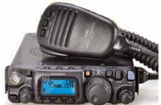
*Yaesu FT-817 HF/VHF/UHF transceiver packs a lot of features into a small space. (Size 5.3" × 1.5" × 6.5").*
