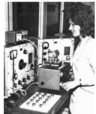
Measurement of ferrite core losses using frequencies up to 1.5 MHz at Mullard's magnetic materials plant in Crossens during the 1970s.
