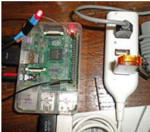
Lovji employed an external 4-port USB hub (right) that only takes up one USB port on the Raspberry Pi 2. [N2CKD pic.]
