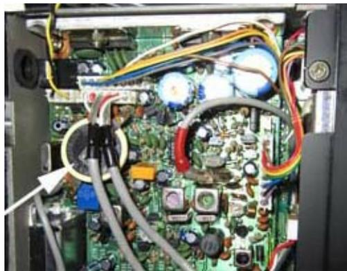
Icom IC-38A 220 MHz FM transceiver with replacement lithium cell (arrowed) soldered to the circuit board for memory backup.
