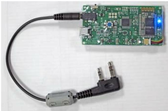
Mike, N2HTT's Mobilinkd Bluetooth KISS TNC for Android phone, with HT interface cable. Unit can run 48 hours from the included 1200 mAh Li-Ion battery.
