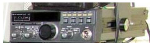
*Yaesu FT-480R (1980) 2 meter SSB/CW/FM transceiver relies on the vehicle battery for memory backup.*
