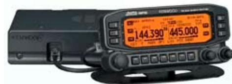
*Kenwood TM-D710G dual-band FM transceiver has built-in TNC and GPS for mobile APRS operation.*
