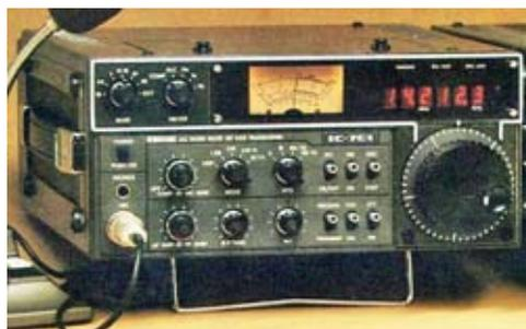
*Icom IC-701/IC-710 (1976) was one of the earliest amateur radio transceivers with digital synthesis.*
