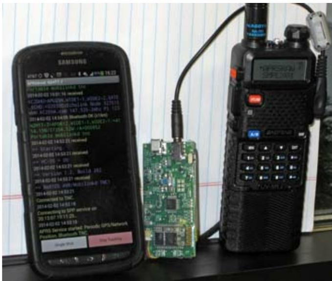
N2HTT portable APRS setup with (L to R) Samsung Galaxy S4 smartphone, Mobilinkd Bluetooth TNC, connected to the BaoFeng UV-5R dual-band FM transceiver. Smartphone screen shows received packets.
