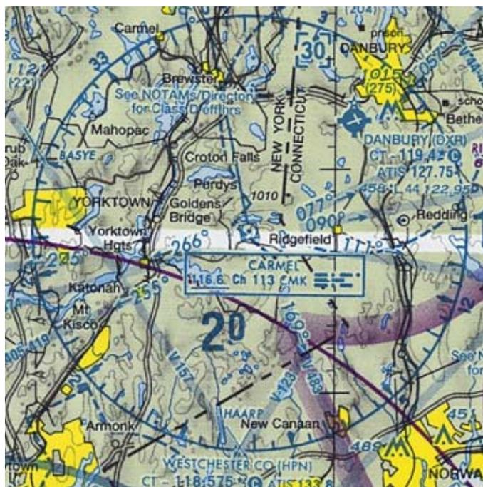
*FAA Aeronautical Chart shows location of VOR/DME beacon **CMK**, along with the frequency 116.6 MHz and dots and dashes of the Ident.*
