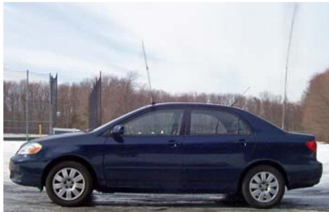
*N2KZ / mobile now boasts an optimized 2-element directional array with a dual band 2 meter/440 antenna on the roof and Hustler CGT-144 2 meter antenna on the trunk.*
