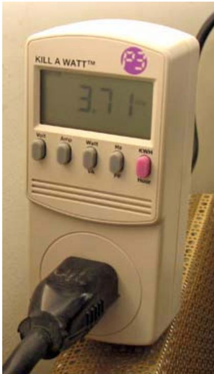
P3 International's "Kill A Watt" power meter displays volts, amps, watts and kWh.
