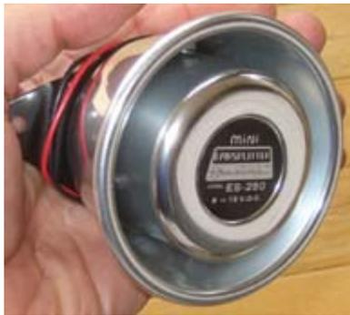
*Kolin Mini Earsplitter Model ES-250 from 1975 emitted an 85 dB yelping sound when supplied with 6 - 12 volts DC. It was completely transistorized, with no moving parts.*
