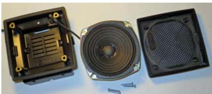
View inside a Motorola HSN4018B mobile loudspeaker.
