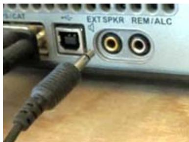
Many radios have a 1/8 inch jack socket for an external speaker.
