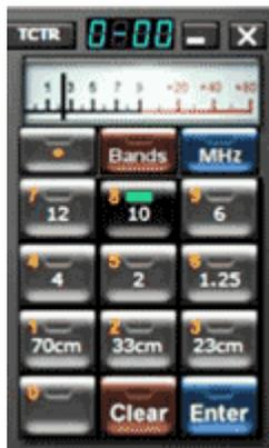
*S-meter and band-framing buttons.*
