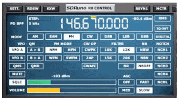
SDRuno software’s “RX CONTROL” window for adjustment of frequency, mode, filter bandwidth, squelch etc.
