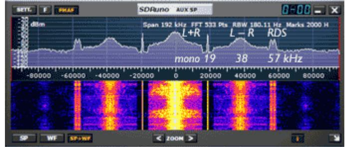
AUX SP (Auxiliary spectrum) window shows demodulated signal from FM broadcast station WFUV, 90.7 MHz. Clearly visible are the mono (L+R) signal, 19 kHz pilot tone, stereo difference signal (L–R) modulated onto a 38 kHz carrier (suppressed) and RDS data at 57 kHz.
