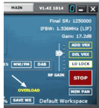
*Yellow “OVERLOAD” indicator (arrowed) in the “MAIN” window can be fixed by reducing RF GAIN.*
