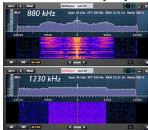
*“AUX SP” display for AM broadcast station WCBS, 880 kHz (top) shows conventional upper and lower sidebands compared with all-digital ‘blocks’ for HD Radio station WFAS, 1230 kHz.*
