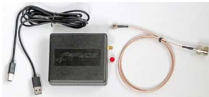
*RSP1A with USB 2.0 A-B cable (left) and SMA male to SO-239 female cable.*
