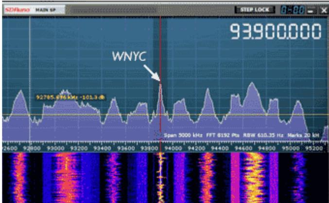
Part of the “MAIN SP” display showing FM broadcast stations between 92.7 and 95.1 MHz. At the time, WNYC was in analog mono with its HD Radio digital sidebands visible.
