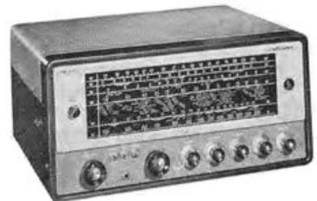
*Hallicrafter SX-62A as featured in the 'Guide to Short Wave Listening'. Priced just under \$400 in 1961 it covered three short wave bands from 1.62 to 32 MHz, plus FM or AM from 27 to 109 MHz.*
