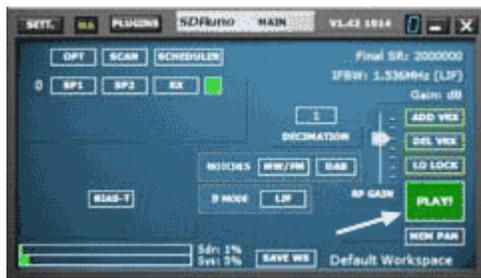
Nothing will happen until you press the “PLAY!” button (arrowed) in the “MAIN” window of SDRuno.
