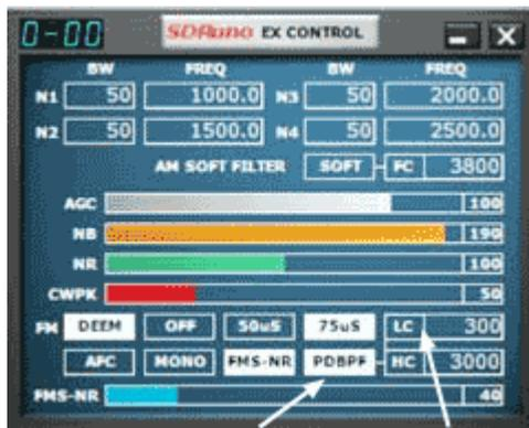
*“EX CONTROL” window provides extra controls for the receiver — including the “PDBF” filter with adjustable low cut (LC).*
