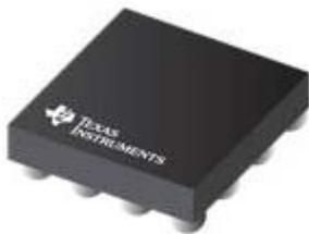
*Texas Instruments TAS2557 5.7-W Class-D audio amplifier with class-H boost, speaker sense and TI SmartAmp speaker protection.*
