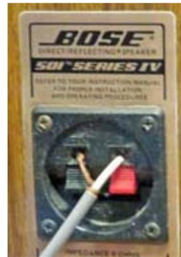
Shielded audio cable feeding a Bose loudspeaker.
