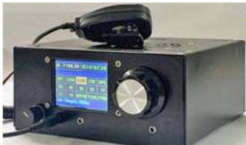
The Arduino-controlled  $\mu$ BITX v6 is shown installed in HF Signals' laser-cut, powder coated aluminum case.
