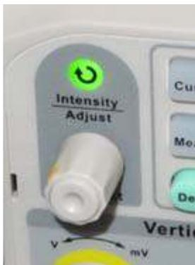
Front panel Intensity/Adjust knob is used to modify all sorts of values in the on-screen menu system.
