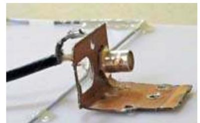
BNC connector is mounted on a metal bracket.
