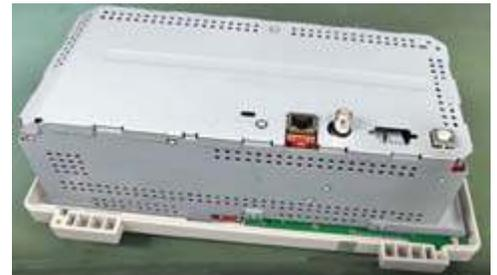
*Metal chassis under the Siglent 'scope's plastic case provides adequate shielding.*
