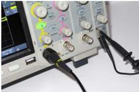
*Test probe is wired into Channel 1 BNC socket with probe clips connected to the front panel square wave output terminals.*
