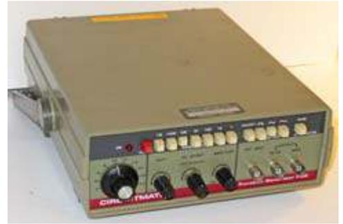
Beckman Circuitmate FG2 function generator covers 0.2 Hz to 2.0 MHz.
