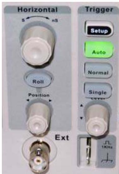
Horizontal timebase and trigger controls for SDS1202X-E.
