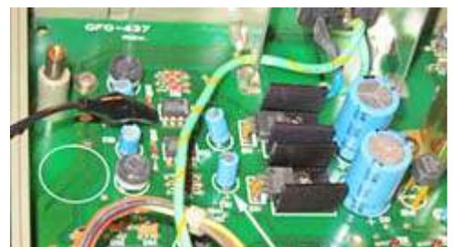
C107 (arrowed), Luxon 47 $\mu$ F electrolytic capacitor had to be replaced in the FG2.
