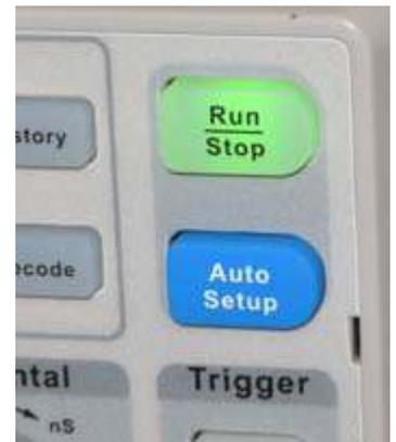
Auto Setup and Run/Stop buttons are top-right on the front panel.
