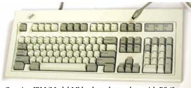
*Genuine IBM ‘Model M’ keyboard complete with PS/2 mini-DIN connector. Do **not** use this type of keyboard!*
