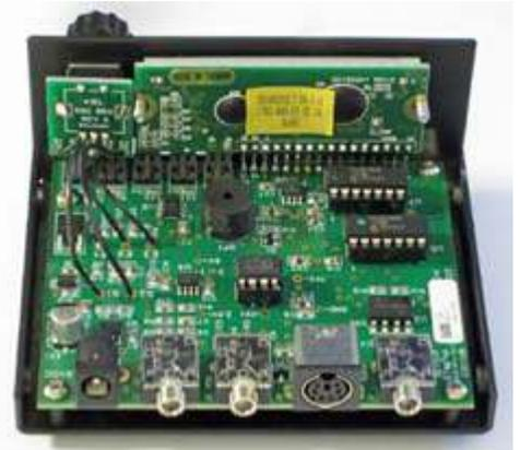
*Main circuit board and LCD board mounted in the metal enclosure ready for initial testing.*
