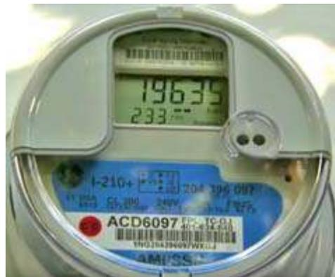
GE/Silver Spring smart meter in operation. Item to right of LCD is the IR optical port.
