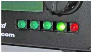
*Five LEDs need careful alignment to fit through the front panel.*
